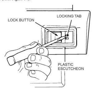
Figure 14 Door Lock Button Escutcheon Removal
