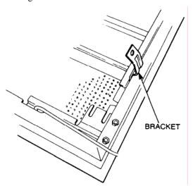
Figure 21 Window Glass Removal
