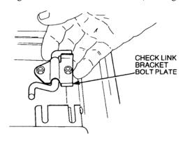
Figure 19 Check Link Bracket Removal
