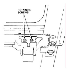
Figure 25 Interior Door Lock Button Removal
