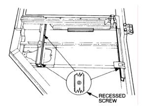
Figure 20 Window Channel Screws Removal
