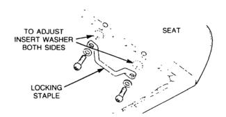
Figure 10 Rear Seat Locking Staple Replacement
