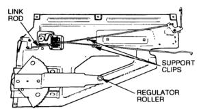
Figure 16 Rear Side Door Inner Panel Removal
