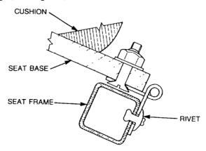
Figure 9 Rear Seat Hinge Replacement
