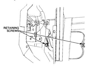
Figure 18 Rear Door Lock Removal
