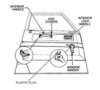
Figure 13 Window Winder Handle Removal
