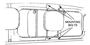
Figure 11 Rear Seat Centre Head Restraint Removal
