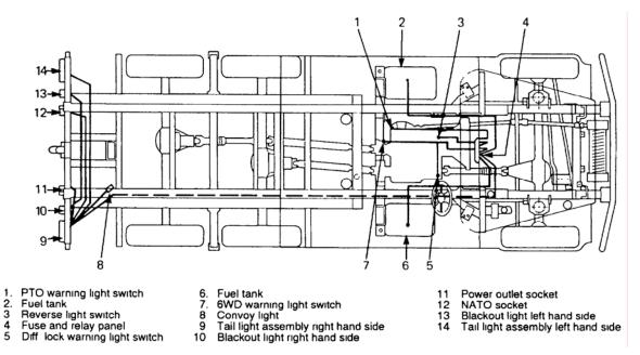
Figure 5 Rear Wiring Harnesses
