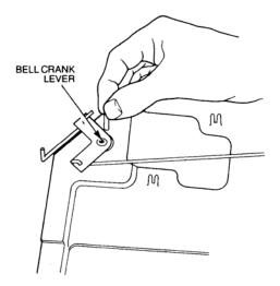
Figure 17 Link Rod Bell Crank Pivot Removal
