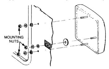
Figure 12 Rear Seat Side Head Restraint Replacement
