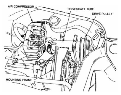
Figure 2 Air Compressor Removal
