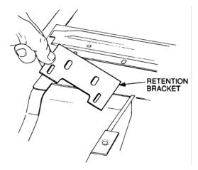
Figure 23 Quarter Window Retaining Bracket
