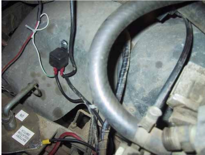
Figure 4 Engine Bay Mounting Location for the New Relay
