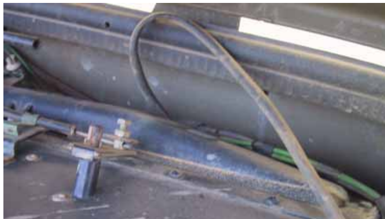
Figure 3 12-volt Ignition Wire – Engine Bay End
