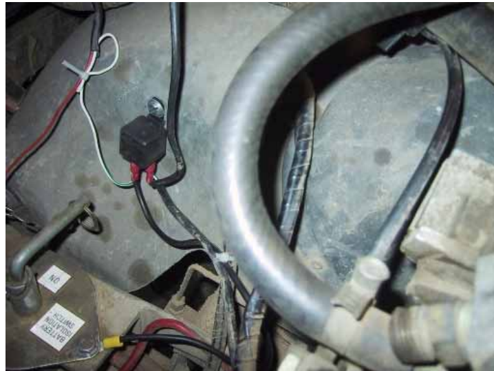
Figure 7 Engine Bay Mounting Location for the New Relay
