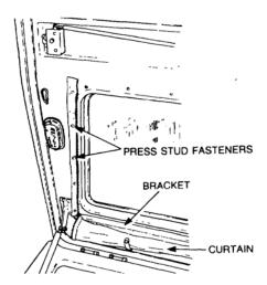
Figure 39 Rear Door Curtain Removal
