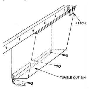
Figure 40 Tumble Out Bins Removal
