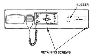
Figure 21 Auxiliary Switch Panel Removal
