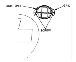
Figure 11 Scan Light Protective Grid Removal
