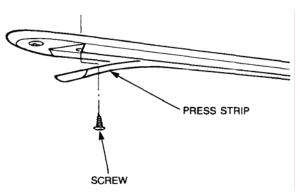
Figure 20 Communication Switch Removal
