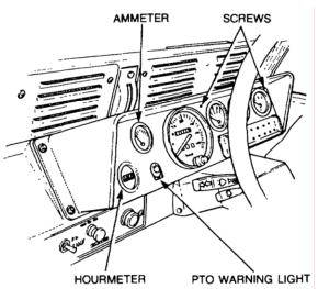
Figure 7 Instrument Panel Removal
