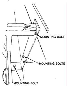
Figure 44 Litter Frame Removal
