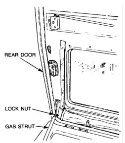
Figure 31 Upper Gas Strut Mounting Removal
