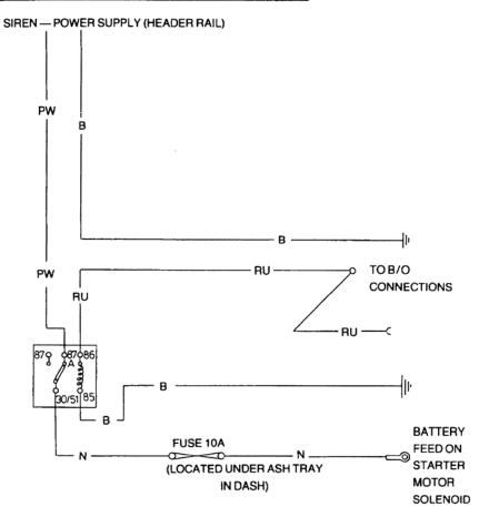
Figure 47 Siren Power Supply Circuit
