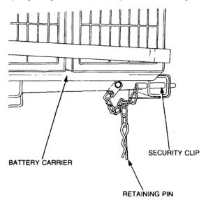
Figure 6 Battery Compartment
