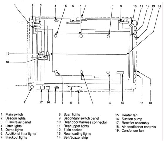
Figure 4 Rear Wiring Harnesses (Ambulance)
