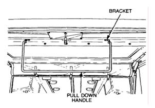
Figure 28 Rear Door Pull Down Handle Removal
