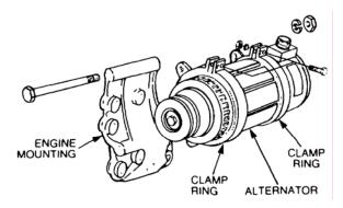
Figure 3 Alternator Installation
