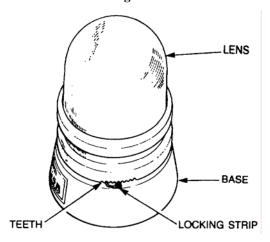
Figure 14 Rotating Beacon Light Lens Removal
