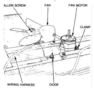
Figure 46 Condenser Motor Fan Removal
