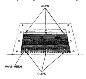
Figure 45 Condenser Wire Mesh Removal
