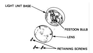
Figure 16 High Level Lights (Rear Door) Bulb Replacement
