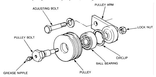
Figure 1 Jockey Pulley Exploded View
