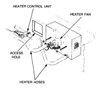
Figure 24 Heater Unit Removal
