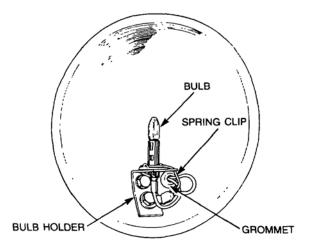
Figure 12 Scan Light Bulb Replacement
