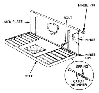
Figure 30 Rear Step Exploded View
