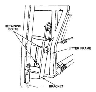
Figure 43 Oxygen Cylinder Bracket Removal
