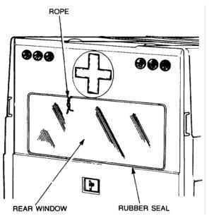
Figure 37 Rear Door - Acrylic Plastic Installation
