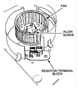
Figure 25 Heater Fan Removal
