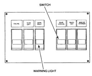
Figure 18 Secondary Switch Panel Removal
