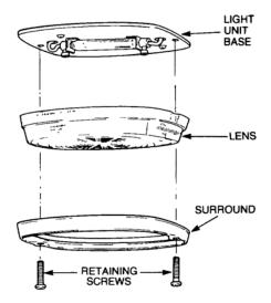
Figure 10 Loading Light Exploded View
