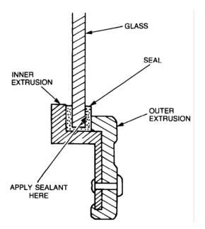
Figure 36 Rear Window Frame – Applying Sealant
