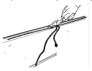
Figure 35 Rubber Seal – Applying Soap Solution
