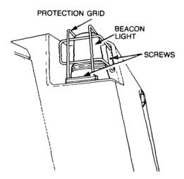
Figure 13 Rotating Beacon Light Grid Removal
