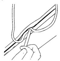
Figure 34 Rubber Seal - Installing Rope
