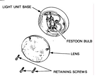
Figure 8 Interior Ceiling Light Bulb Replacement
