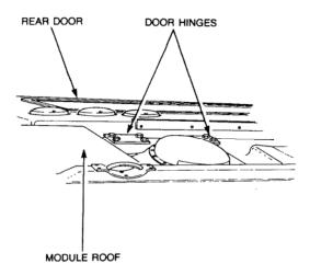
Figure 32 Rear Door Hinge Removal
