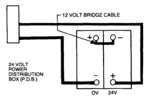
Figure 5 Batteries Installation
