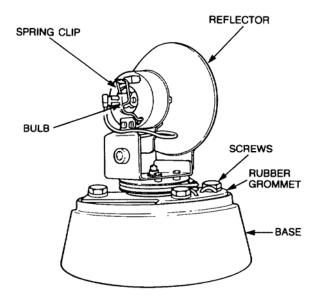
Figure 15 Rotating Beacon Light Bulb Replacement
