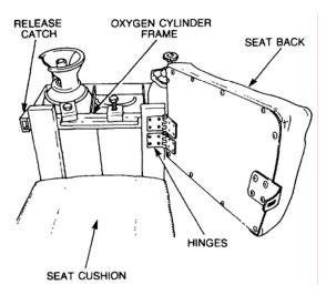
Figure 38 Seat Back Removal
