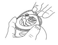
Figure 150 Installing the O ring
