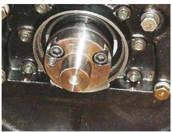
Figure 48 Crank Plate Secured to the Crankshaft
