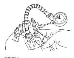
Figure 149 Checking the Journal Bearing Axial Clearance
