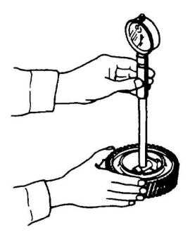
Figure 34 Measuring the Idle Gear
