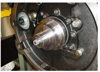
Figure 50 Push Cone Located on Crank Plate and Against Seal
