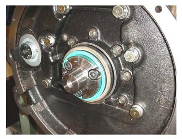
Figure 49 Rear Crankshaft Oil Seal Located on the Crank Plate Ready for Installation
