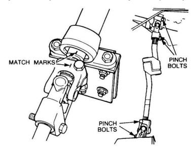
Figure 134 Alignment of the Steering Column
