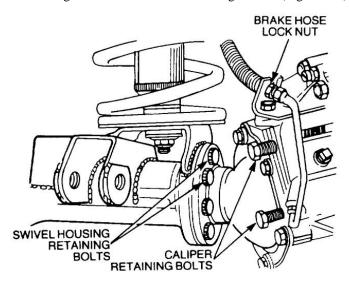
Figure 114 Removal of the Brake Calliper
