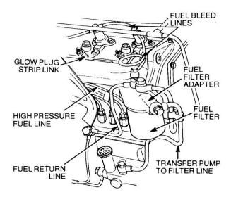
Figure 19 Removal of the Fuel Lines
