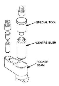
Figure 127 Replacement of the Rocker Beam Centre Bush
