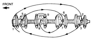
Figure 33 Removal of the Rocker Shaft
