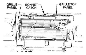
Figure 2 Removal of the Grille Panel
