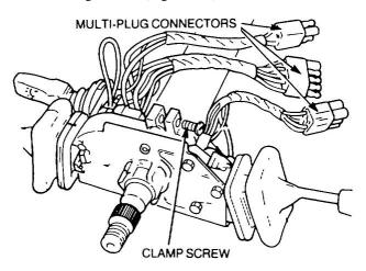
Figure 137 Removal of the Switch Cluster
