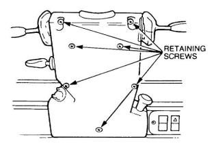
Figure 136 Removal of the Steering Column Shroud
