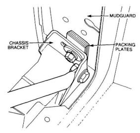
Figure 152 Removal of the Left Mudguard
