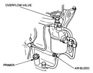
Figure 29 Installation of the Fuel Filter
