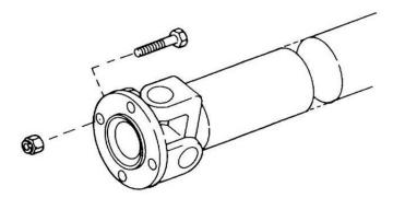
Figure 100 Removal of the Propeller Shaft to Rear Axle Flange
