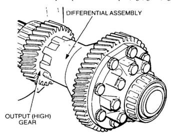
Figure 72 Removal of the Differential Assembly
