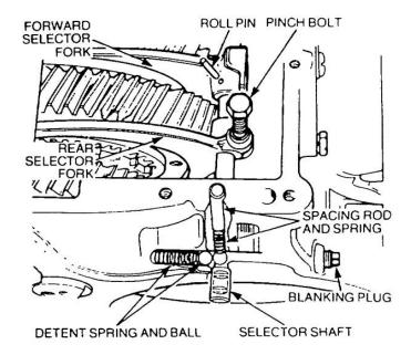
Figure 75 Removal of the Transfer Selectors
