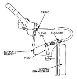
Figure 59 Removal of the Parking Brake Cable
