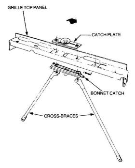
Figure 16 Installation of the Bonnet Catch
