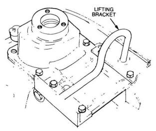
Figure 62 Transmission Lifting Bracket
