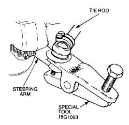
Figure 115 Removal of the Steering Linkage
