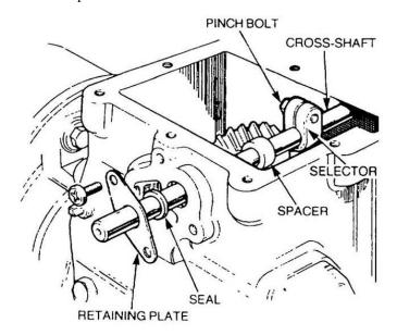
Figure 76 Removal of the Transfer Selector Cross-shaft
