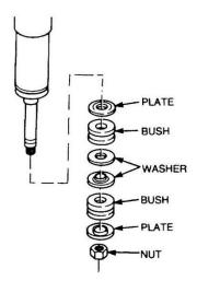
Figure 98 Removal of the Shock Absorber
