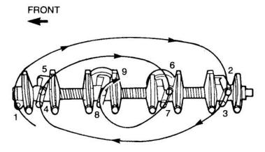
Figure 20 Removal of the Rocker Shaft
