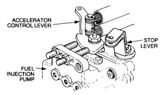
Figure 8 Removal of the Engine Stop Cable
