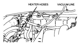
Figure 18 Removal of the Heater Hoses and Vacuum Line
