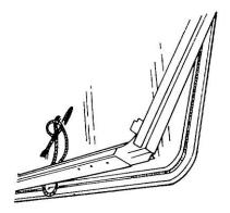
Figure 162 Installation of the Windscreen Glass
