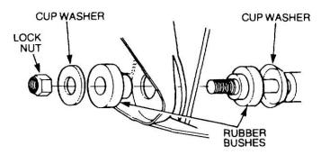
Figure 112 Installation of the Radius Arm Bush
