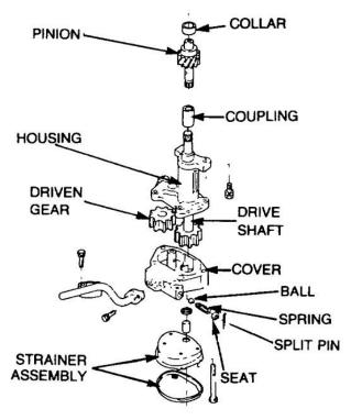
Figure 37 Oil Pump - Exploded View
