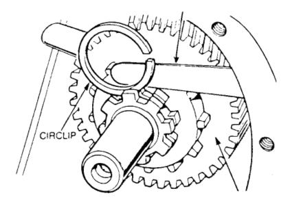
Figure 91 Adjustment of the Mainshaft Pre-load
