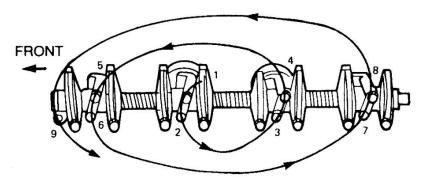
Figure 27 Rocker Shaft Assembly - Tightening Sequence
