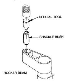
Figure 126 Replacement of the Rocker Beam Spring Bush
