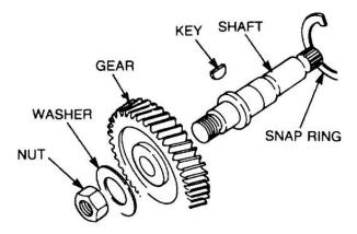
Figure 147 Removal of the Drive Gear
