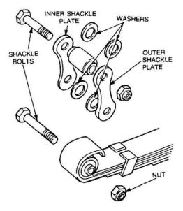
Figure 122 Removal of the Shackle Bolts (Rocker Beam End)
