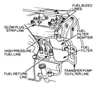
Figure 30 Installation of the Fuel Lines
