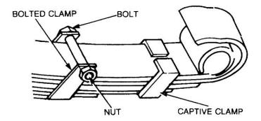
Figure 129 Removal of the Spring Clamps
