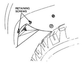
Figure 157 Removal of the Mudguard-to-toe Board Bracket
