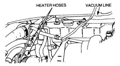
Figure 31 Installation of the Heater Hoses and Vacuum Line
