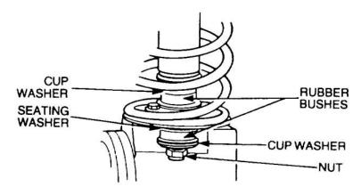
Figure 113 Installation of the Front Shock Absorber
