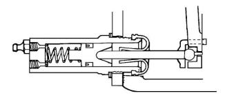
Figure 12 Installation of the Slave Cylinder
