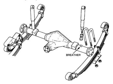
Figure 101 Removal of the Rear Axle Breather
