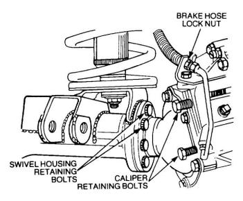
Figure 110 Removal of the Brake Calliper
