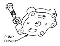
Figure 145 Removal of the Steering Pump Cover
