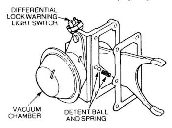
Figure 69 Removal of the Differential Lock Vacuum Chamber Assembly
