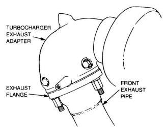
Figure 6 Removal of the Front Exhaust Pipe
