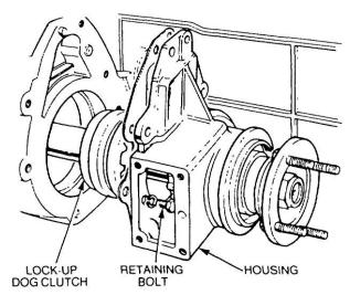
Figure 70 Removal of the Front Output Shaft and Housing
