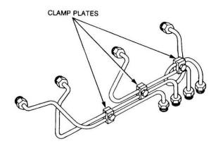
Figure 28 Clamp Plate Location
