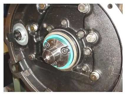
Figure 49 New Type of Seal (Placed on Crank Plate Ready for Installation)
