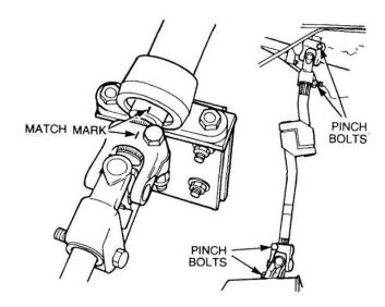
Figure 131 Alignment of the Steering Column
