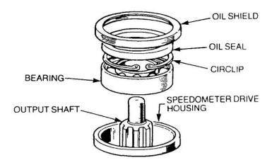
Figure 71 Removal of the Output Shaft
