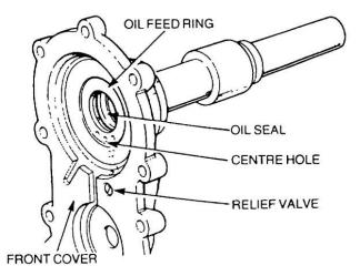
Figure 84 Installation of the Oil Feed Ring and Relief Valve
