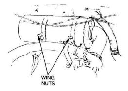
Figure 56 Removal of the Air Cleaner
