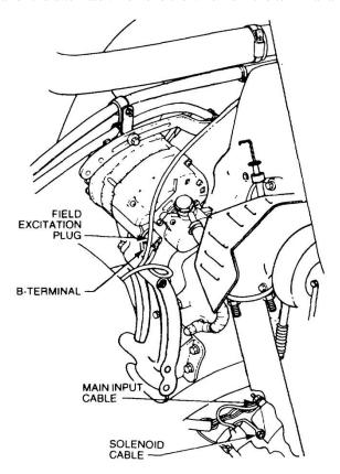
Figure 9 Removal of the Alternator and Starter Motor Cables
