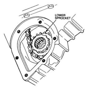
Figure 88 Removal of the PTO Chain
