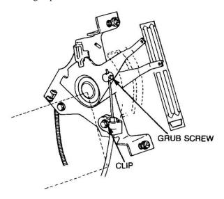
Figure 163 Removal of the Heater Assembly
