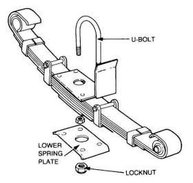
Figure 120 Removal of the U-Bolt and Retaining Plate
