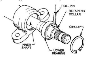
Figure 140 Removal of the Inner Shaft and Bearing
