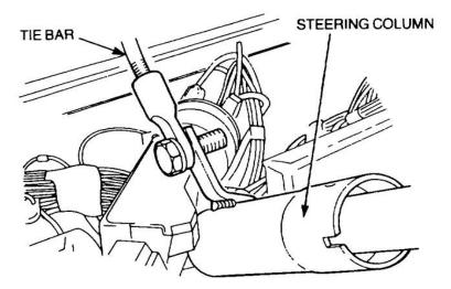
Figure 135 Disconnection of the Steering Column Tie Bar
