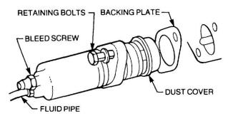
Figure 10 Removal of the Slave Cylinder
