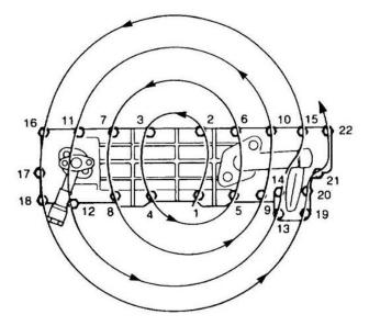
Figure 42 Oil Cooler - Tightening Sequence
