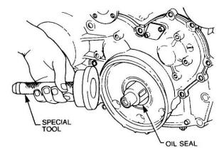
Figure 47 Installation of the Crankshaft Front Oil Seal
