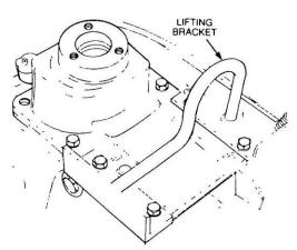
Figure 55 Transmission Lifting Bracket
