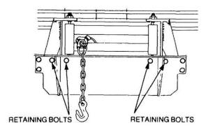
Figure 168 Removal of the Fairlead Frame to Winch Housing
