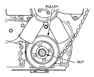
Figure 46 Removal of the Crankshaft Pulley
