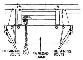
Figure 167 Removal of the Fairlead Frame to the Chassis
