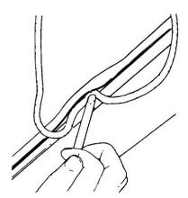
Figure 159 Installing Rope into the Rubber Seal
