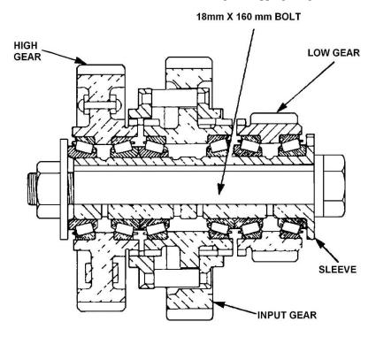
Figure 78 Intermediate Gear Assembly Pre-load Adjustment – Sectional View
