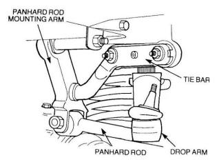
Figure 132 Removal of the Tie Bar
