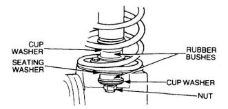
Figure 109 Removal of the Front Shock Absorber
