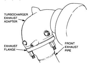
Figure 57 Removal of the Front Exhaust Pipe
