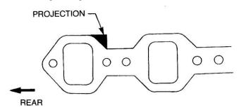
Figure 25 Installation of the Inlet Manifold Gasket
