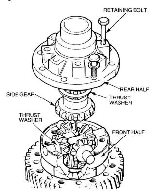
Figure 77 Reassembly of the Differential
