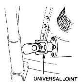
Figure 166 Disconnection of the Winch Input Shaft Universal Joint
