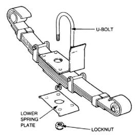
Figure 103 Removal of the U-Bolt
