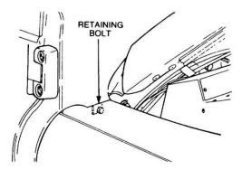
Figure 156 Removal of the Mudguard-to-firewall Bracket
