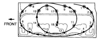
Figure 21 Removal of the Cylinder Head Bolts
