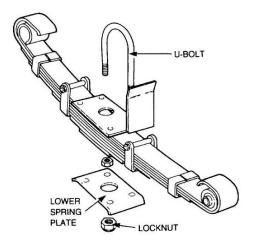
Figure 99 Removal of the U-Bolt
