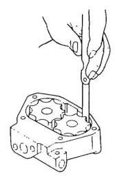
Figure 41 Checking the Gear to Cover Clearance
