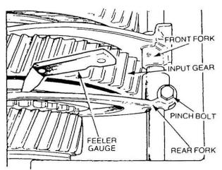
Figure 80 Adjustment of the Transfer Selectors
