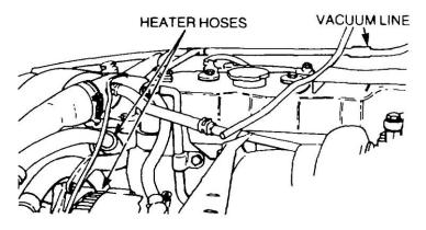
Figure 3 Removal of the Heater Hoses
