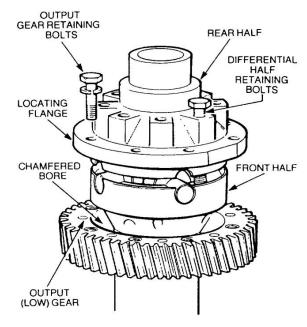
Figure 73 Removal of the Output (Low) Gear
