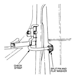
Figure 158 Removal of the Door
