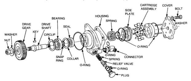
Figure 143 Disassembly of the Power Steering Pump
