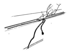
Figure 160 Applying Soap Solution to the Rubber Seal
