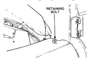
Figure 153 Removal of the Mudguard-to-firewall Bracket
