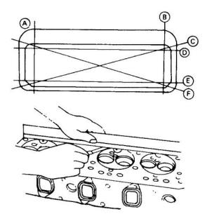
Figure 22 Checking for Cylinder Head Distortion
