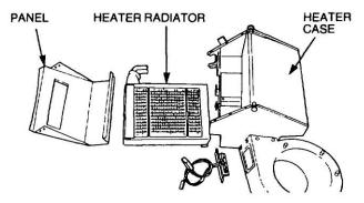
Figure 165 Heater Assembly - Exploded View
