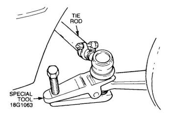
Figure 107 Removal of the Tie Rod
