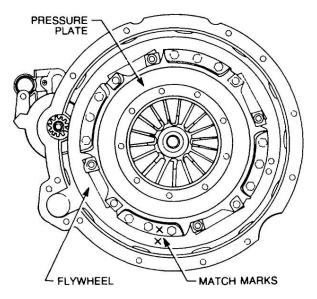
Figure 51 Removal of the Pressure Plate
