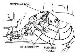
Figure 130 Removal of the Flexible Hoses to the Steering Box
