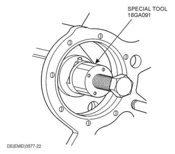
Figure 89 Removal of the Transfer Gear and Spacer
