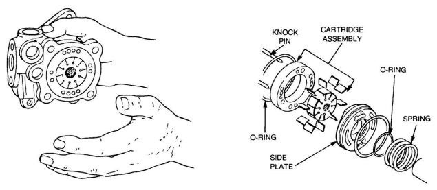
Figure 146 Removal of the Cartridge and Coil Spring
