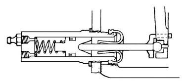
Figure 63 Installation of the Slave Cylinder
