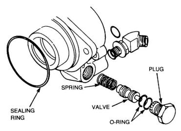
Figure 144 Removal of the Flow Control Assembly
