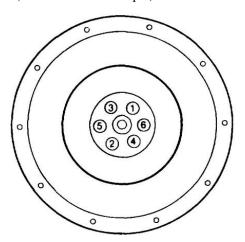
Figure 45 Flywheel - Tightening Sequence
