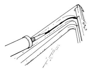
Figure 161 Applying Sealant to the Windscreen Frame
