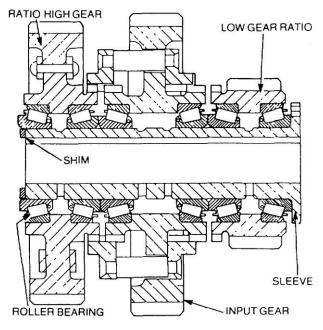
Figure 68 Intermediate Gears - Sectional View
