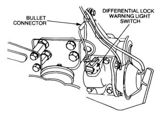
Figure 64 Connection of the Differential Lock
