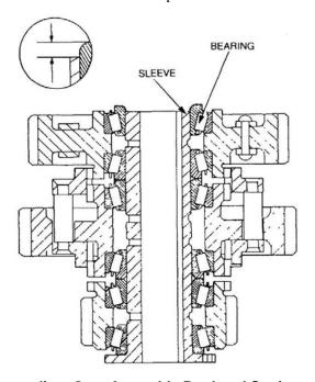
Figure 79 Intermediate Gear Assembly Pre-Load Setting - Sectional View
