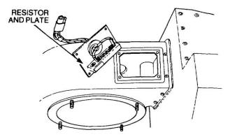
Figure 164 Removal of the Resistor and Plate
