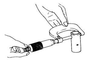
Figure 35 Camshaft Follower Outside Diameter Dimensions
