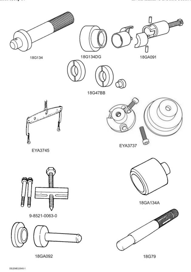
Figure 1 Special Tools (Sheet 1 of 2)
