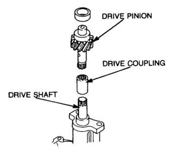
Figure 38 Removal of the Drive Pinion, Collar and Coupling
