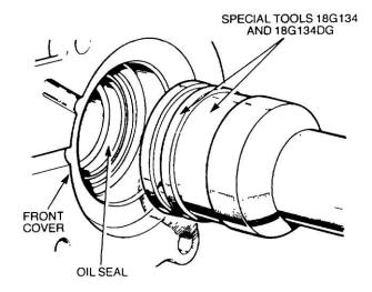
Figure 83 Installation of the Front Cover Oil Seal
