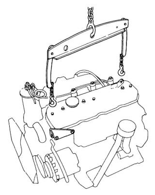
Figure 11 Removal of the Engine
