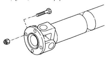
Figure 96 Removal of the Intermediate Axle Flange to Propeller Shaft
