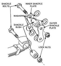
Figure 119 Removal of the Shackle Bolts (Rocker Beam End)
