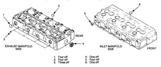
Figure 44 Cylinder Head Expansion Plug Location
