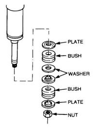
Figure 102 Removal of the Shock Absorber
