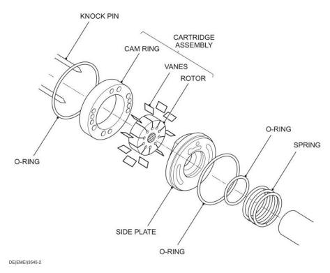
Figure 150 Power Steering Pump - Exploded View
