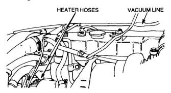
Figure 15 Vacuum Line and Heater Hose Connections
