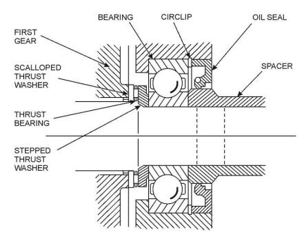
Figure 90 Installation of the Seal and Rear Spacer
