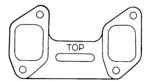
Figure 23 Installation of the Exhaust Manifold Gasket
