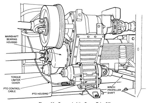
Figure 66 Removal of the Power Take-Off
