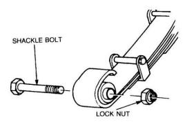
Figure 121 Removal of the Shackle Bolt (Fixed End)
