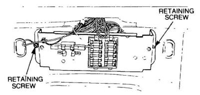
Figure 53 Removal of the Fuse Box
