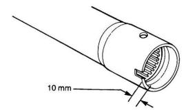
Figure 142 Installation of the Upper Column Bearing
