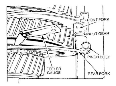
Figure 92 Selector Fork Adjustment
