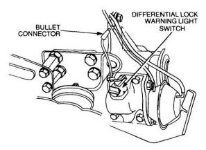
Figure 58 Disconnection of the Differential Lock
