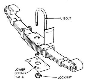
Figure 123 Removal of the U-Bolt And Retaining Plate
