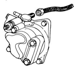
Figure 5 Removal of the Pump-to-power Steering Hoses
