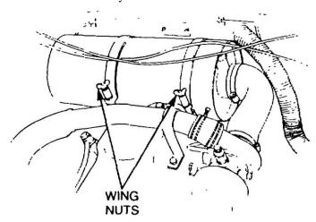
Figure 4 Removal of the Air Cleaner
