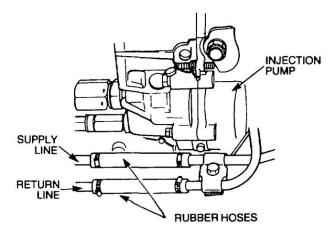
Figure 14 Installation of the Fuel Lines
