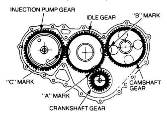
Figure 36 Aligning the Gear Timing Marks
