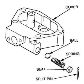
Figure 39 Removal of the Oil Relief Valve Ball
