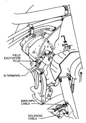
Figure 13 Installation of the Alternator and Starter Motor Cables
