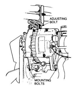
Figure 32 Alternator Adjusting Bolts
