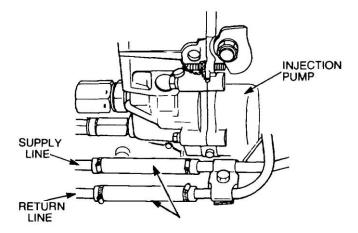
Figure 7 Removal of the Fuel Lines
