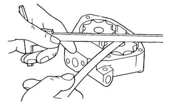
Figure 40 Checking the Gear to Body Clearance
