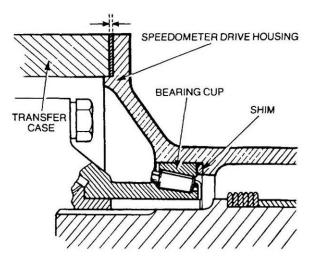
Figure 81 Differential Assembly - Pre-Load Adjustment - Sectional View
