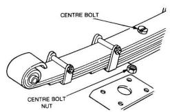
Figure 128 Replacement of the Centre Bolt
