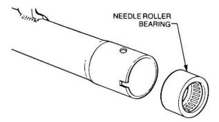
Figure 141 Removal of the Upper Column Bearing
