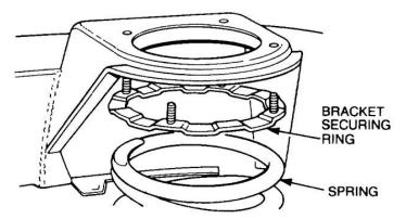
Figure 118 Removal of the Front Spring
