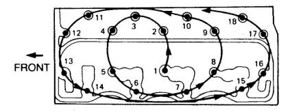
Figure 26 Cylinder Head Bolts - Tightening Sequence
