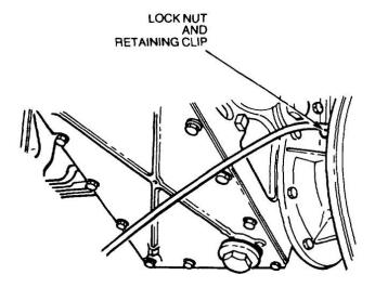
Figure 60 Removal of the Speedometer Cable
