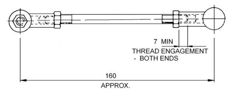
Figure 94 Rod Adjustment
