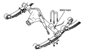
Figure 97 Removal of the Intermediate Axle Breather
