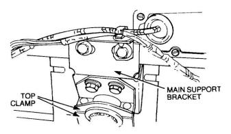
Figure 139 Removal of the Steering Column Upper Mounting
