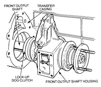
Figure 82 Installation of the Front Output Shaft Housing
