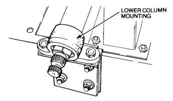
Figure 138 Removal of the Steering Column Lower Mounting
