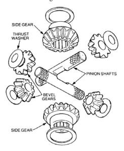
Figure 74 Removal of the Differential Gears
