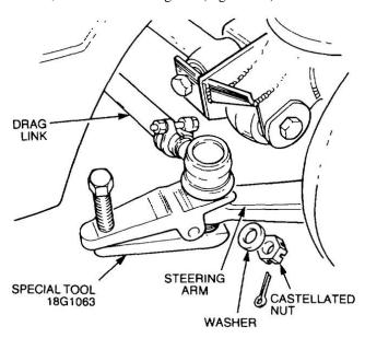
Figure 111 Removal of the Drag Link
