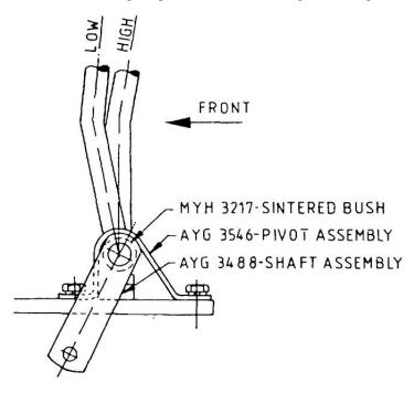
Figure 93 High/Low Range Selector Lever
