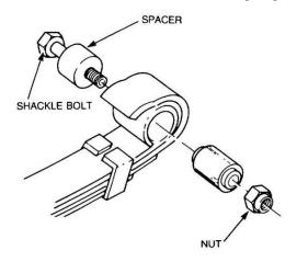
Figure 124 Removal of the Shackle Bolt (Fixed End)
