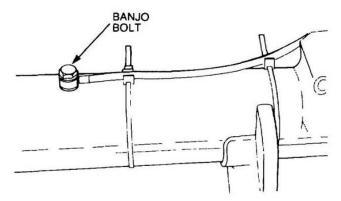
Figure 105 Removal of the Front Axle Breather Hose
