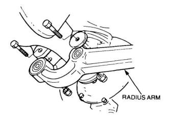
Figure 108 Removal of the Radius Arm
