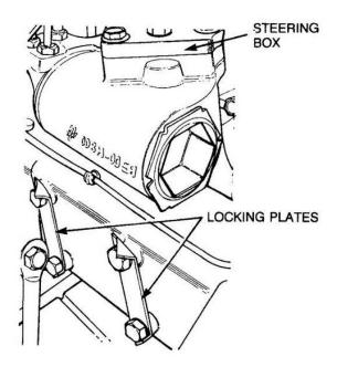
Figure 133 Removal of the Steering Box
