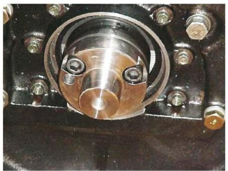
Figure 48 Crank Plate (Secured to Crankshaft)
