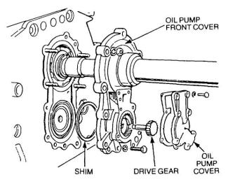
Figure 85 Installation of the Oil Pump Front Cover
