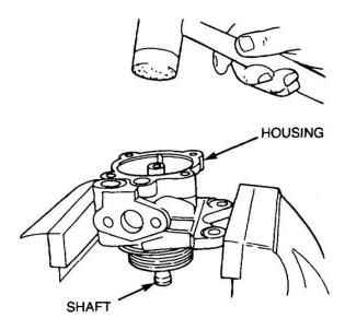
Figure 148 Removal of the Pump Shaft from the Housing
