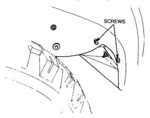
Figure 154 Removal of the Mudguard-to-toe Board Bracket
