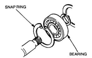
Figure 149 Removal of the Snap Ring and Bearing
