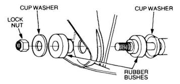
Figure 106 Removal of the Radius Arm Bush
