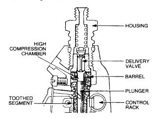
Figure 21 Housing and Delivery Valve Location
