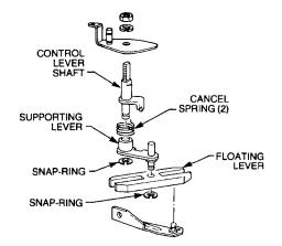
Figure 31 Control Assembly – Exploded View
