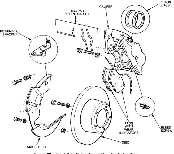
Figure 63 Front Disc Brake Assembly – Exploded View
