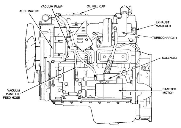
Figure 4 Isuzu Engine 4BDT1, Left-hand Side
