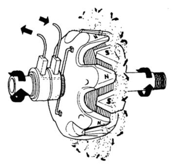
Figure 79 Rotor and Magnetic Field
