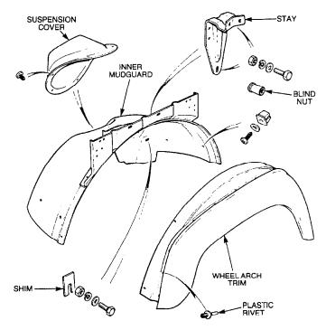
Figure 89 Left-hand Front Inner Mudguard and Wheel Arch Trim - Exploded View
