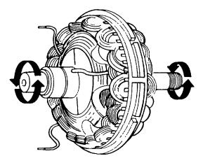
Figure 78 Rotor and Stator Assembly
