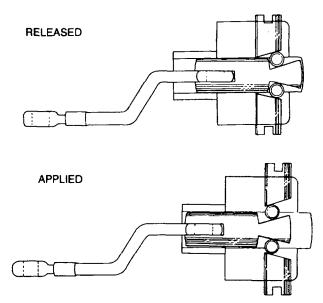
Figure 66 Parking Brake Expander Operation
