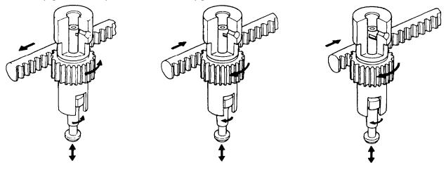
Figure 19 Plunger Rotating Mechanism
