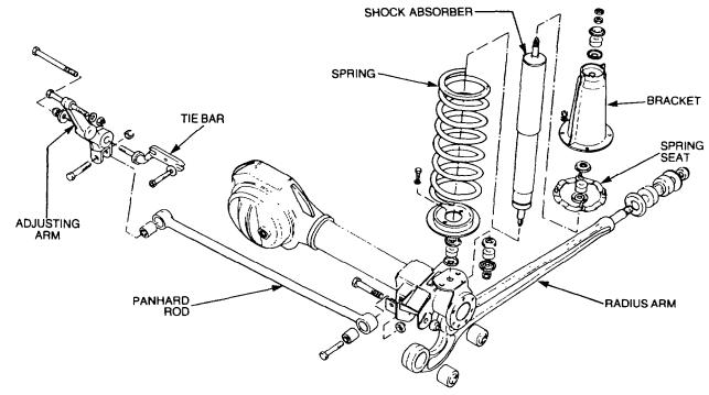
Figure 68 Front Suspension – Left-hand Side
