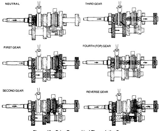
Figure 46 Drive Transmitted Through the Gears
