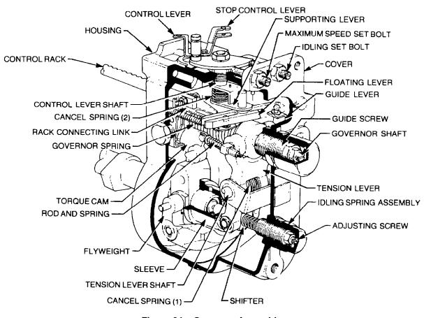
**63.** Figure 24 illustrates the governor assembly showing the location of the various components.
