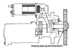
Figure 76 Ignition Switch in START
