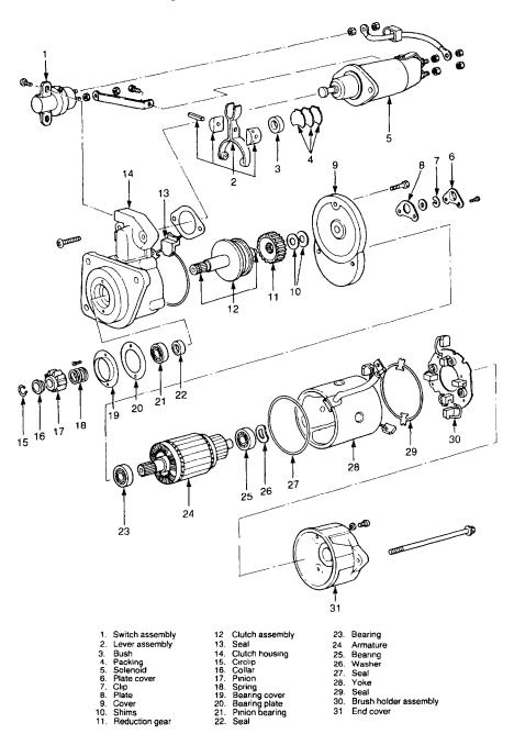
Figure 77 Starter Motor – Exploded View
