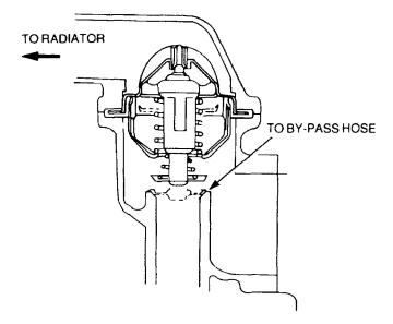
Figure 6 Thermostat Operation
