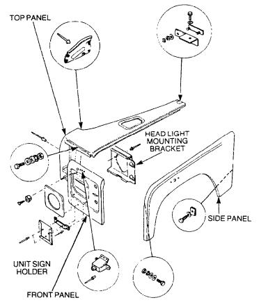
Figure 88 Left-hand Front Outer Mudguard – Exploded View
