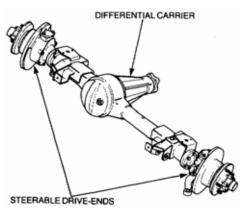
Figure 53 Front Axle Assembly
