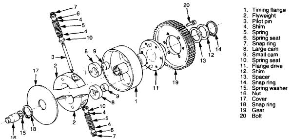
**79.** The automatic timer achieves this function by means of flyweights, springs and eccentric cams (refer to Figure 40).
