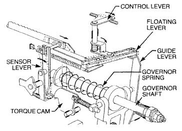
Figure 36 Returning to the Idle Position
