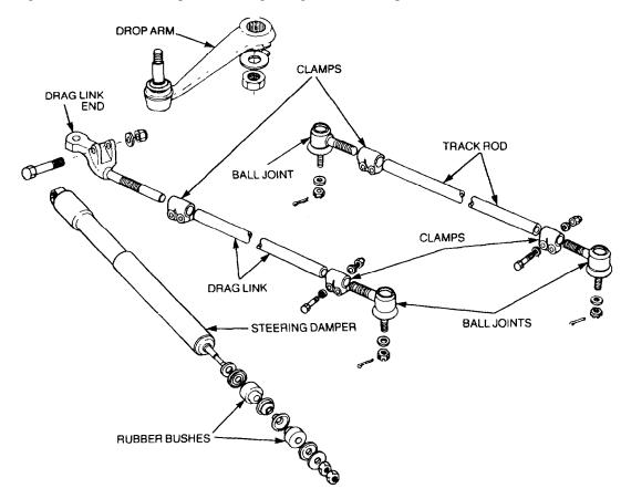
Figure 73 Drop Arm, Steering Linkages and Steering Damper
