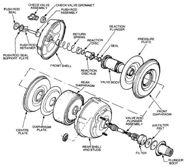
Figure 60 Brake Servo Vacuum Chamber – Exploded View
