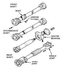
Figure 51 Front, Intermediate and Rear Propeller Shafts
