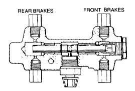
Figure 57 Hydraulic Circuit – Normal Condition
