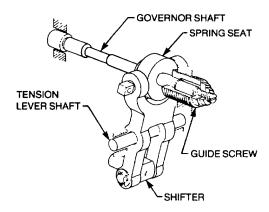
Figure 27 Tension Lever and Governor Shaft
