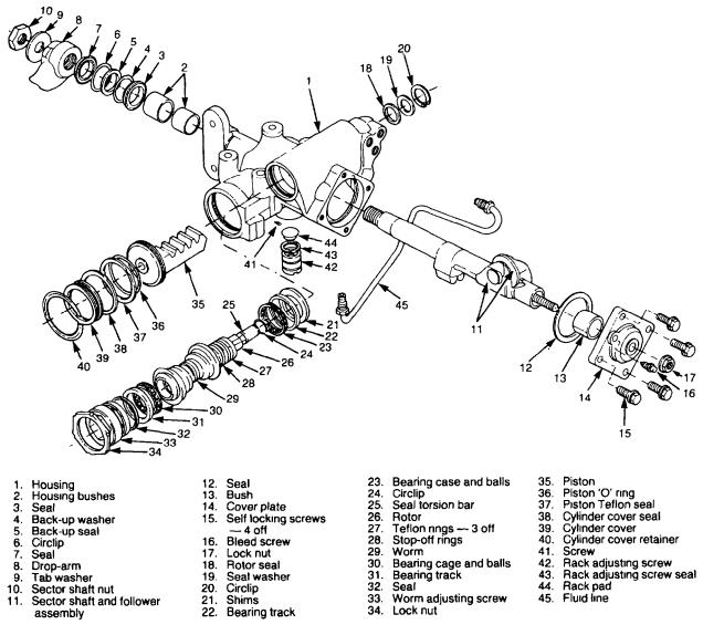
Figure 72 Steering Box Assembly – Exploded View
