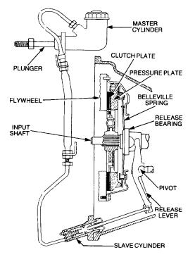
Figure 44 Clutch Assembly – Sectional View
