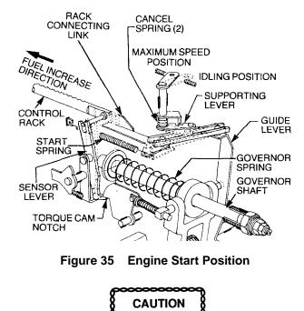
Do not allow the engine to rev up after it starts. This will prevent the sensor lever from disengaging from the notch on the torque cam and dangerously interfering with the governor control of the injection pump.
