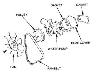
Figure 7 Water Pump Assembly
