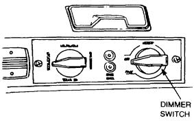
Figure 81 Lighting Control Switch Location
