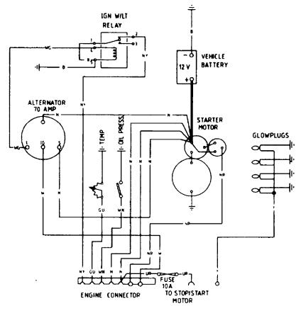
Figure 74 Engine Electrical Circuit
