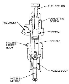
Figure 23 Fuel Injector Assembly
