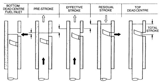
Figure 22 Phases (Strokes) of the Plunger
