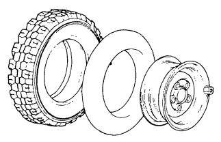
Figure 2 Tyre, Tube and Rim
