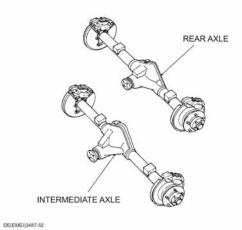
Figure 52 Intermediate and Rear Axle Assemblies
