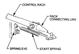
Figure 30 Connecting Link and Start Spring Location
