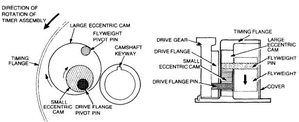
Figure 41 Automatic Timer – Static Position
