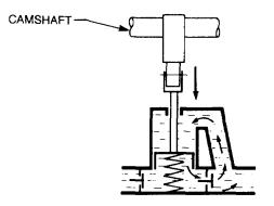
Figure 14 Discharge Stroke
