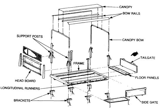
Figure 91 Rear Body – Exploded View
