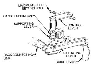
Figure 34 Control Lever Assembly Operation
