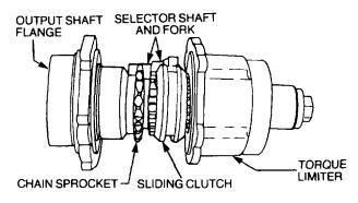
Figure 49 PTO and Torque Limiter Assembly
