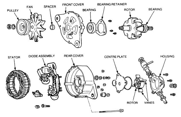
Figure 80 Alternator and Vacuum Pump – Exploded View
