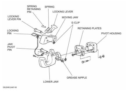
Figure 85 Towing Pintle – Exploded View
