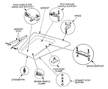
Figure 87 Bonnet and De-ditching Tool Holders – Exploded View
