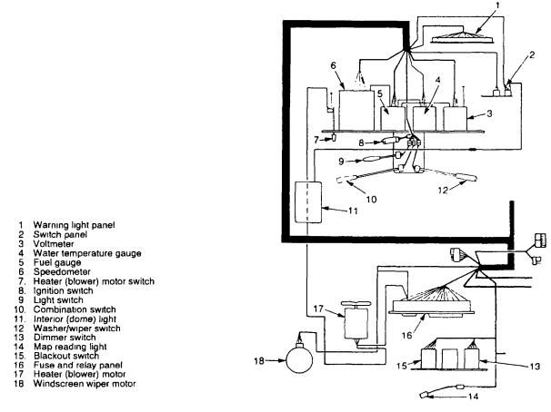
Figure 84 Cabin Wiring
