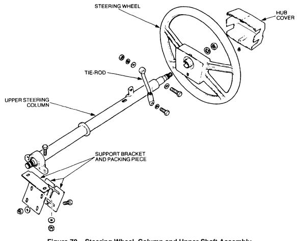
Figure 70 Steering Wheel, Column and Upper Shaft Assembly
