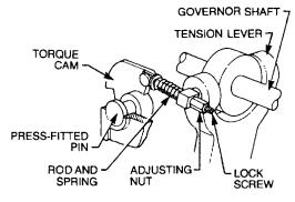
Figure 32 Torque Cam Location
