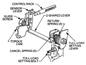
Figure 33 Full-load Setting Lever and Sensor Lever Locations
