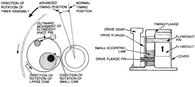
Figure 42 Flyweights in Timing Advance Position
