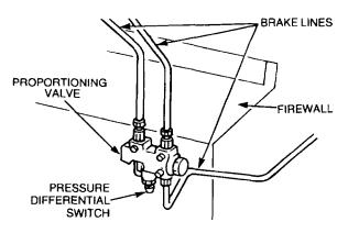
Figure 56 Pressure Differential Switch – Location
