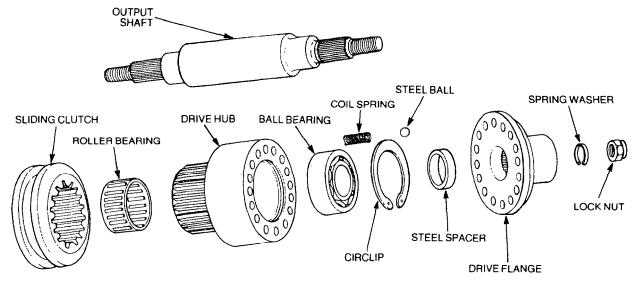
Figure 50 Torque Limiter and Output Shaft – Exploded View
