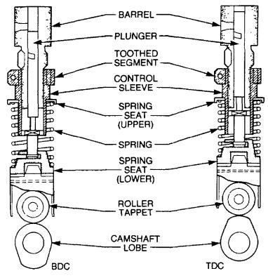
Figure 20 Plunger Drive Assembly
