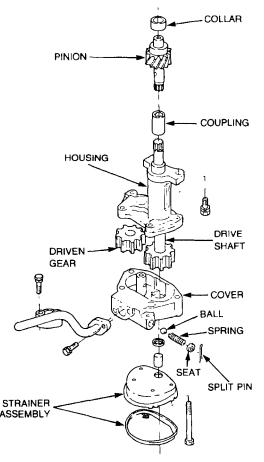
Figure 5 Oil Pump – Exploded View
