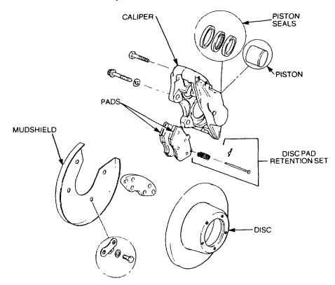
Figure 64 Rear Disc Brake Assembly – Exploded View
