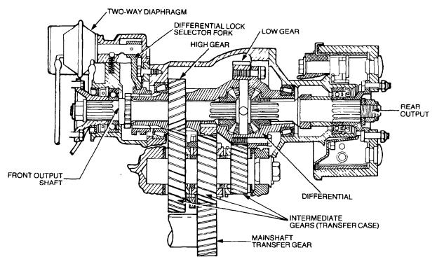
Figure 47 Transfer Case and Differential – Sectional View
