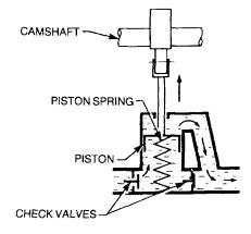
Figure 13 Intake Stroke
