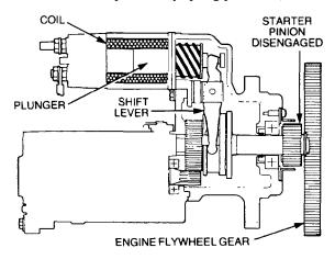
Figure 75 Ignition Switch OFF
