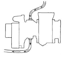
Figure 8 Cooling System – Coolant Flow
