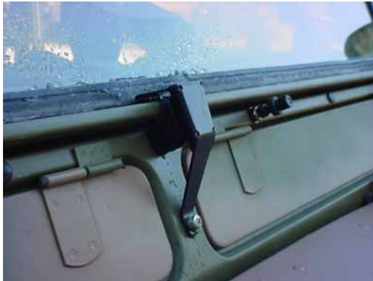
Figure 2 Installed Windscreen Washer Guard
