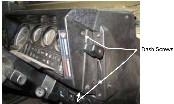
Figure 3 Partially Removed Dash
