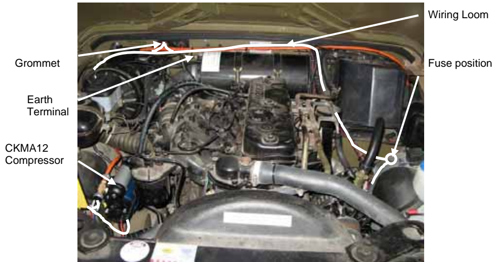
Figure 12 Engine Bay Wiring Loom
