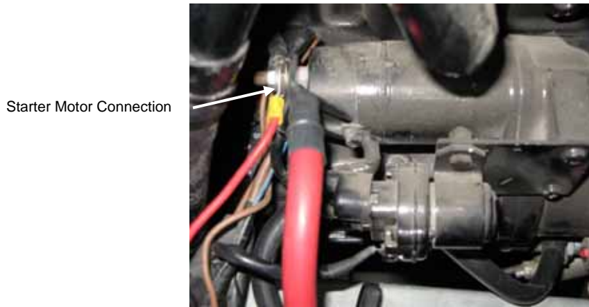
Figure 6 Starter Motor Terminal
