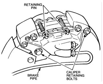
Figure 3 Brake Caliper Removal
