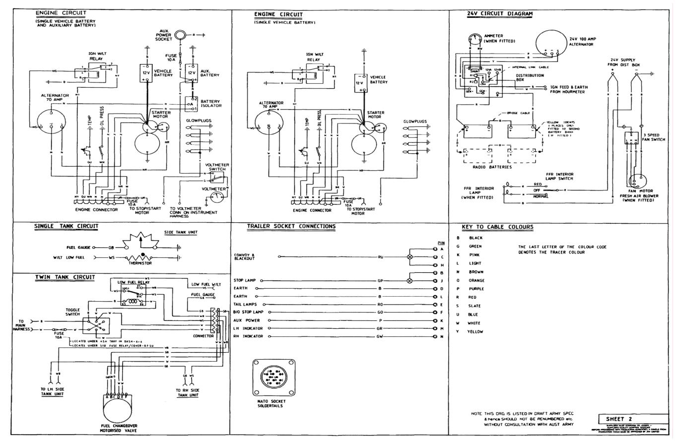
Figure 13 Wiring Diagram (Sheet 2 of 3)
