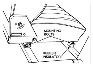
Figure 12 Rear Seat Mounting Bolts
