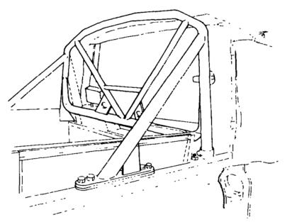
Figure 11 Front Roll Bar Removal
