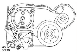
Figure 9 Power Steering Pump Removal
