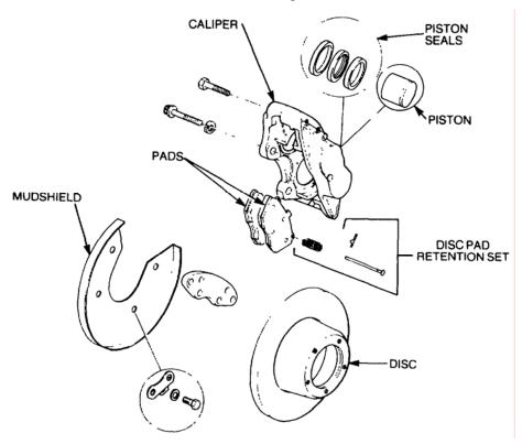
Figure 5 Brake Caliper Exploded View
