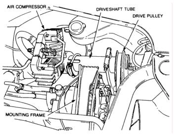
Figure 2 Air Compressor Removal
