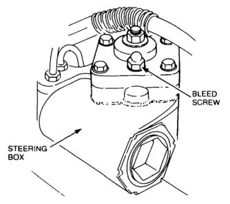
Figure 8 Power Steering Bleed Screw Location
