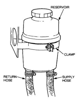
Figure 7 Return And Supply Hoses To Reservoir Removal
