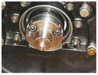
Figure 47 Crank Plate Secured to Crankshaft
