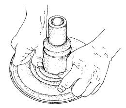
Figure 270 Installing the Front Diaphragm
