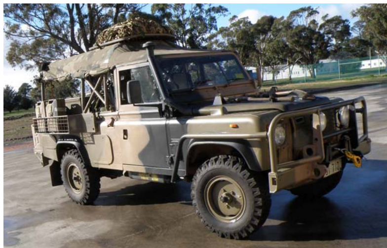
Figure 1 Truck, Surveillance, Lightweight, W/Winch, W/Side stowage, W/Rear seat, MC2 – Land Rover 110 4x4
