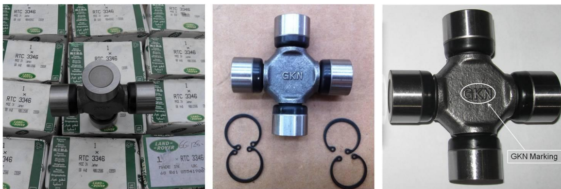
Figure 9 LRA (GKN) Universal Joint and Packaging - NIIN 99-731-0894 / LRA PNo. RTC3346
