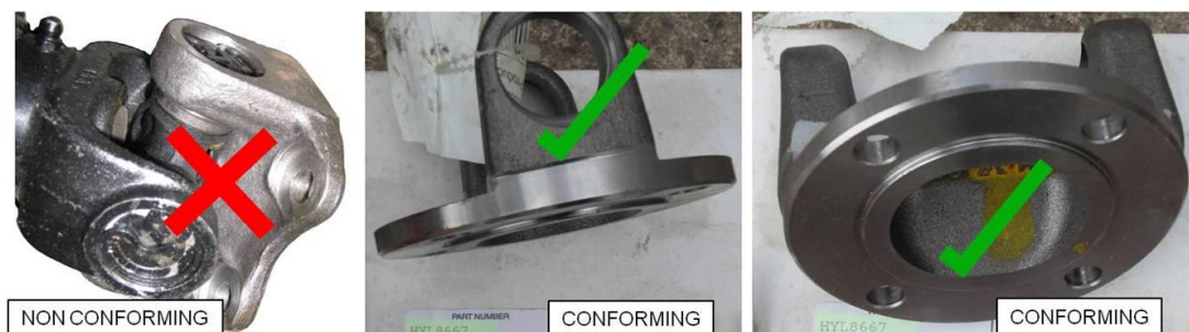
Figure 5 Cast Flange (Non-Conforming) and Forged Steel Flange (Conforming)
