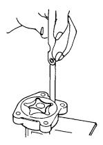
Figure 32 Checking the Outer Rotor to Housing Clearance
