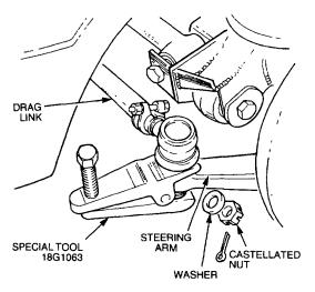
Figure 75 Drag Link Removal
