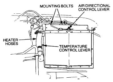
Figure 108 Heater Assembly Removal
