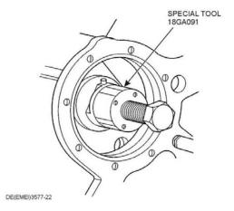
Figure 57 Transfer Gear and Spacer – Removal
