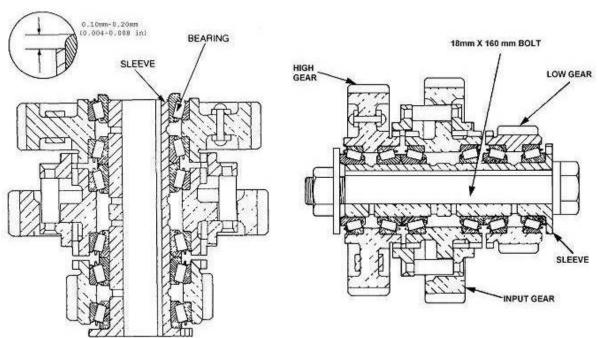
Figure 65 Intermediate Gear Assembly Preload Adjustment and Shim Selection
