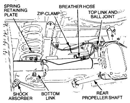
Figure 66 Rear Axle Removal
