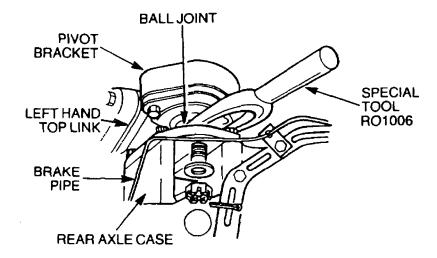
Figure 68 Top Link and Ball Joint Removal
