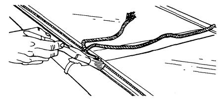
Figure 103 Rubber Seal Applying Soap Solution
