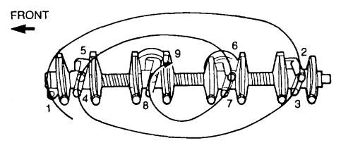
Figure 15 Rocker Shaft - Removal
