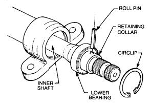
Figure 89 Inner Shaft and Bearing Removal
