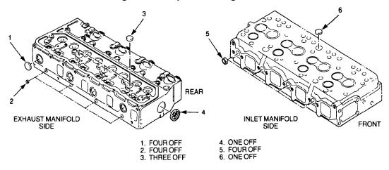
Figure 35 Expansion Plug Location - Cylinder Head
