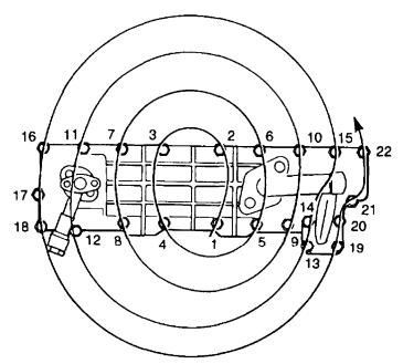
Figure 33 Oil Cooler - Tightening Sequence
