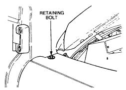
Figure 98 Mudguard to Firewall Removal
