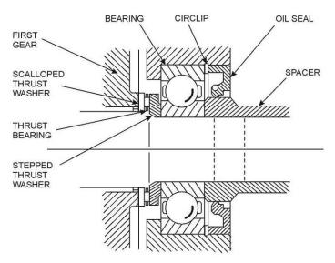
Figure 58 Seal and Rear Spacer - Installation
