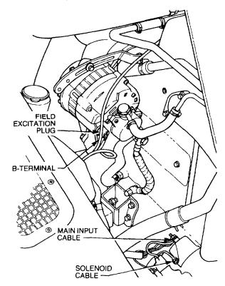
Figure 8 Alternator and Starter Motor Cables
