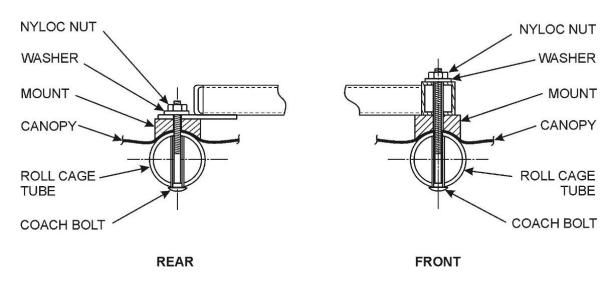
Figure 107 ROPS / RCB Repair Procedure
