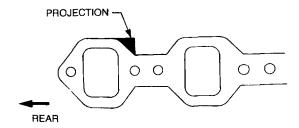
Figure 20 Inlet Manifold Gasket Installation
