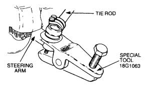
Figure 77 Steering Linkage Removal
