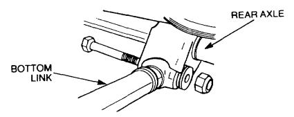
Figure 67 Bottom Link to Axle Bracket
