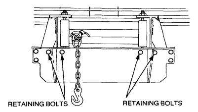
Figure 113 Fairlead Frame Removal
