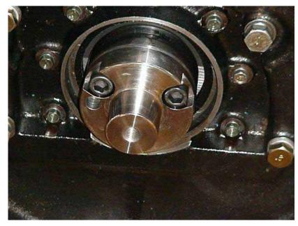
Figure 40 Crank Plate (Secured to Crankshaft)
