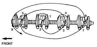
Figure 22 Rocker Shaft Assembly Tightening Sequence
