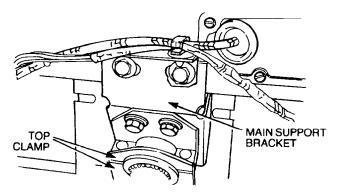
Figure 88 Steering Column Upper Mounting
