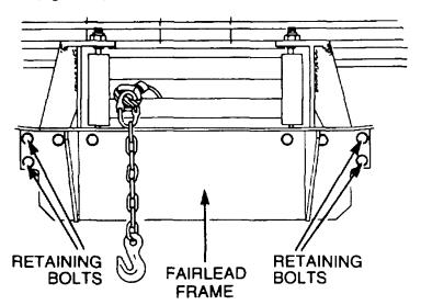
Figure 112 Winch and Fairlead Frame Removal
