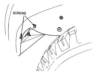
Figure 99 Mudguard to Toe Board Removal
