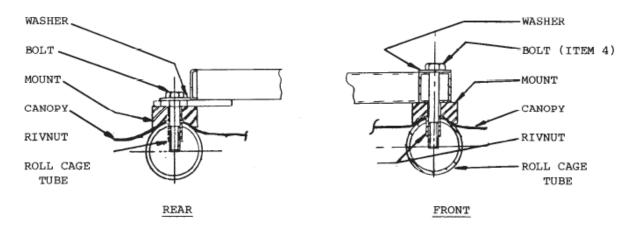
Figure 106 Location of Fixing Components (Using rivnuts)
