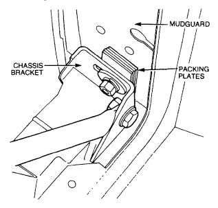
Figure 94 Left Mudguard Mounting
