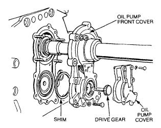
Figure 56 Oil Pump Front Cover Installation
