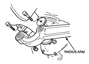
Figure 73 Radius Arm Removal
