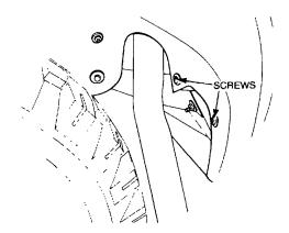
Figure 96 Mudguard-to-toe Board Removal
