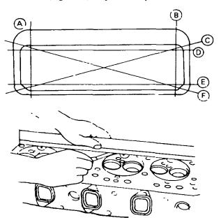
Figure 17 Checking Cylinder Head Distortion
