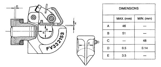
Figure 92 Towing Pintle Wear Limits
