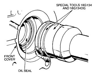
Figure 54 Front Cover Oil Seal Installation
