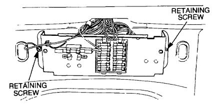
Figure 45 Fuse Box Removal
