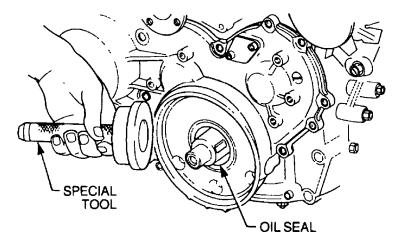
Figure 38 Crankshaft Front Oil Seal Installation
