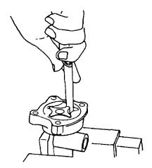
Figure 31 Checking Inner to Outer Rotor Clearance
