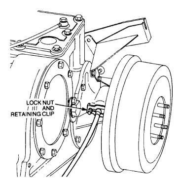
Figure 50 Speedometer Cable Removal
