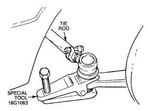
Figure 72 Tie Rod Removal
