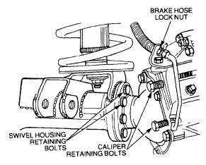
Figure 76 Brake Calliper Removal
