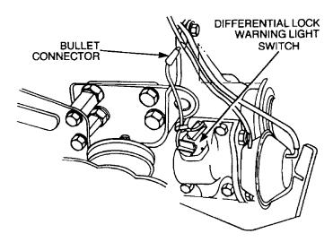
Figure 48 Differential Lock Disconnection
