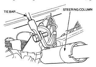
Figure 84 Steering Column Tie Bar Disconnection
