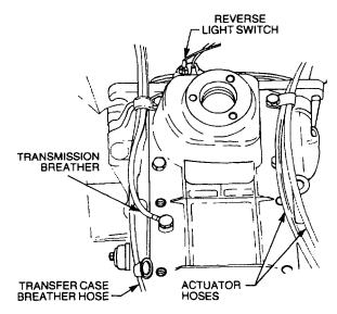
Figure 46 Hose Clamps Removal
