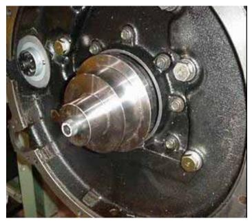
Figure 42 Push Cone (Located on Crank Plate and Against the Seal)
