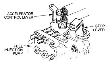
Figure 7 Accelerator Control and Stop Levers
