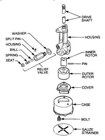
Figure 29 Oil Pump - Exploded View
