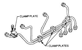
Figure 23 Clamp Plate Location
