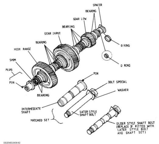
Figure 62 Intermediate Gear Assembly
