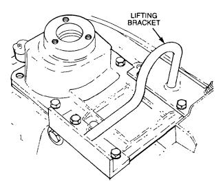
Figure 47 Transmission Lifting Bracket
