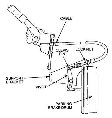
Figure 49 Parking Brake Cable Removal
