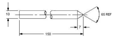
Figure 63 Coupling Pin Punch
