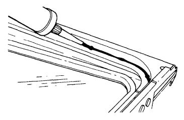
Figure 104 Windscreen Frame Applying Sealant
