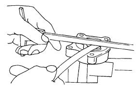
Figure 30 Checking Rotor to Cover Clearance
