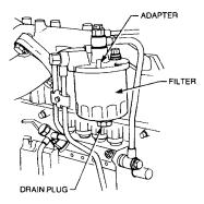
Figure 24 Fuel Filter Installation
