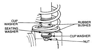
Figure 74 Front Shock Absorber Mounting
