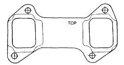
Figure 18 Exhaust Manifold Gasket Installation
