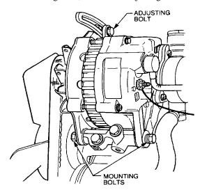
Figure 25 Alternator Adjusting Bolts
