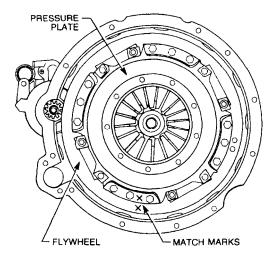
Figure 43 Pressure Plate Removal
