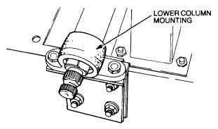
Figure 87 Steering Column Lower Mounting
