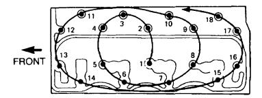
Figure 21 Cylinder Head Bolts Tightening Sequence
