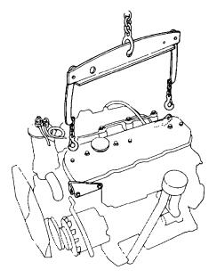
Figure 10 Engine Lifting
