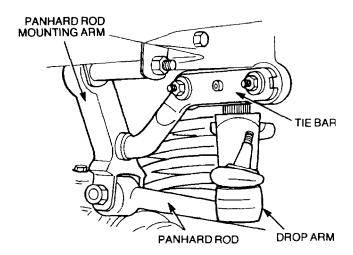
Figure 83 Tie Bar Removal
