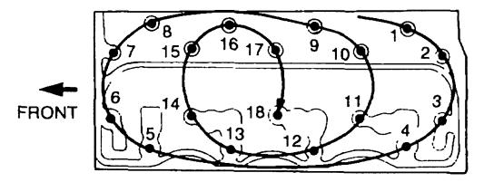
Figure 16 Cylinder Head Bolts - Removal
