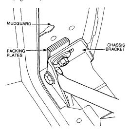
Figure 97 Right Mudguard Mounting
