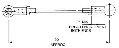
Figure 61 Rod Adjustment
