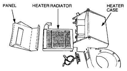
Figure 110 Heater Assembly Exploded View
