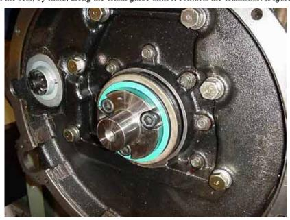
Figure 41 New Type of Seal (Placed on Crank Plate Ready for Installation)
