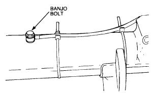
Figure 70 Front Axle Breather Hose Removal
