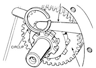
Figure 59 Mainshaft Preload Adjustment
