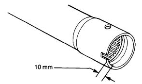
Figure 91 Upper Column Bearing Installation
