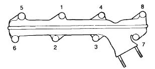
Figure 19 Exhaust Manifold - Tightening Sequence
