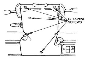
Figure 85 Steering Column Shroud Mounting
