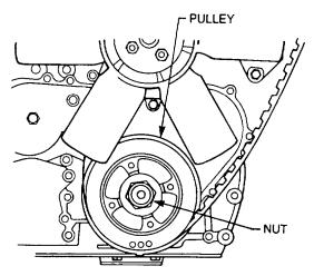
Figure 37 Crankshaft Pulley - Removal
