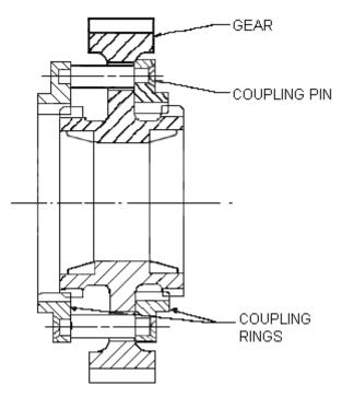
Figure 64 Input Gear Coupling Assembly
