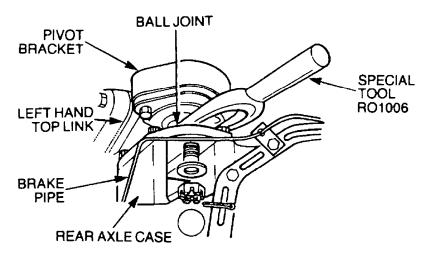
Figure 81 Pivot Bracket Ball Joint Removal
