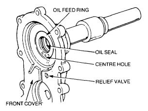
Figure 55 Oil Feed Ring and Relief Valve Installation
