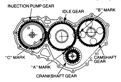
Figure 28 Aligning the Gear Timing Marks
