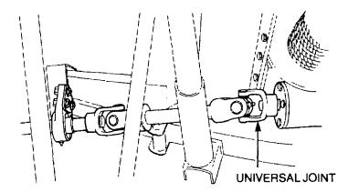
Figure 111 Winch Input Shaft Universal Joint Disconnection
