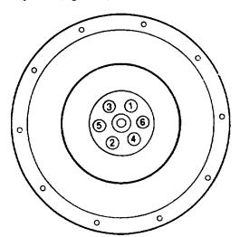
Figure 36 Flywheel - Tightening Sequence
