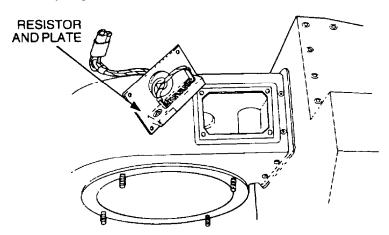
Figure 109 Resistor and Plate Removal
