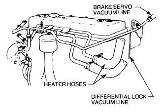
Figure 3 Vacuum Line and Heater Hose Connections
