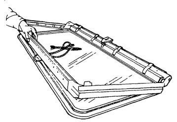
Figure 105 Windscreen Frame Installation
