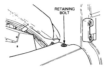
Figure 95 Mudguard-to-firewall Removal
