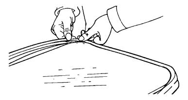
Figure 101 Windscreen Rubber Seal Installation
