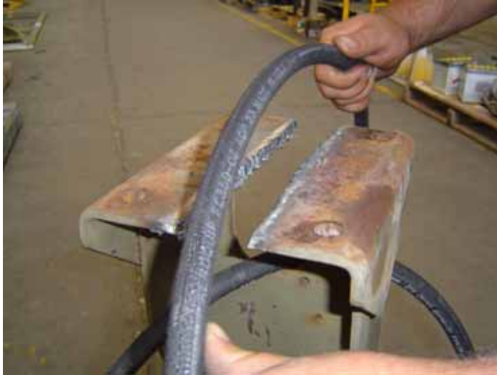
Figure 15 Removing the Fuel Lines.
