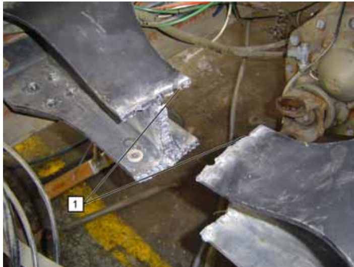
1. Bracket mounting holes
