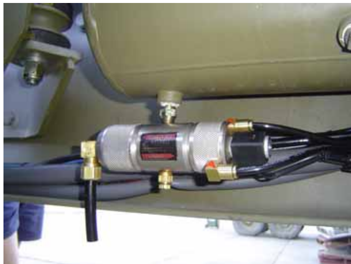
Figure 5 Wet Tank Installation
