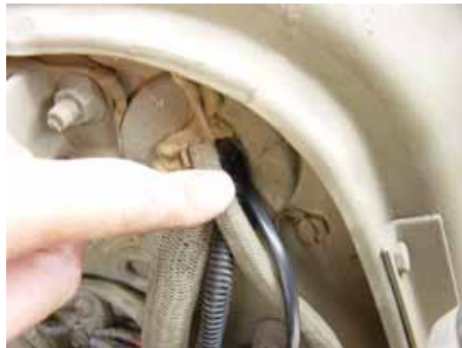
Figure 7 Wiring Harness Entry Point
