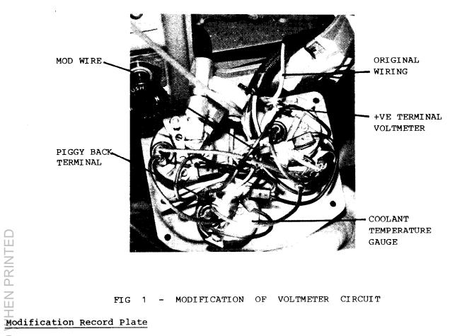
FIG 1 - MODIFICATION OF VOLTMETER CIRCUIT
