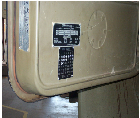
Figure 1 – Modification Plate Location
