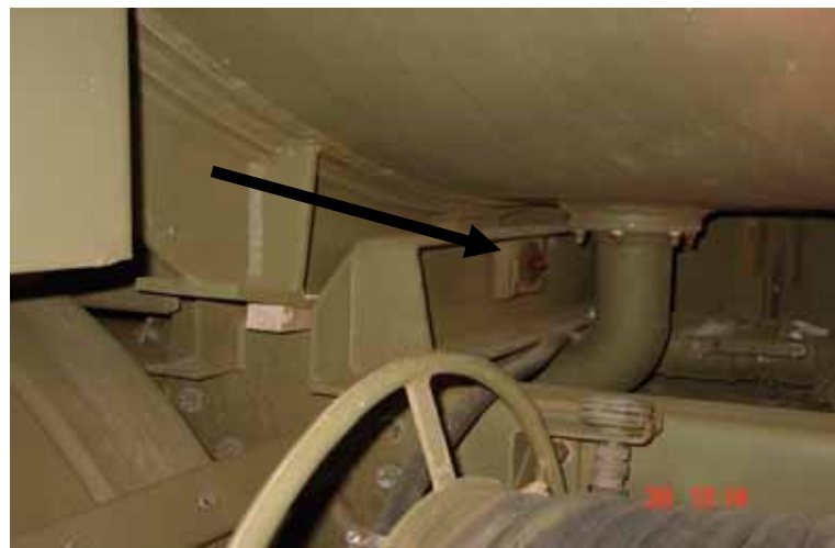
Figure 4 Grease the Rear Mount via the Grease Nipple
