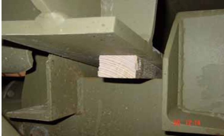
Figure 1 Wooden Wedge – Between Tank Saddle and Tank Mount Passenger Side
