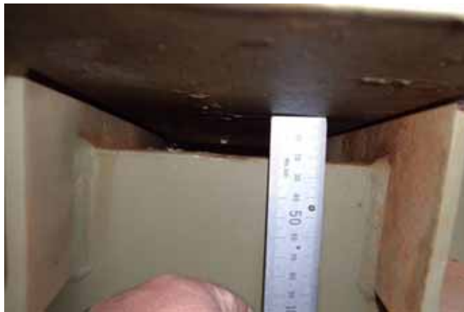
Figure 2 Measuring and Recording the Gap – Driver Side
