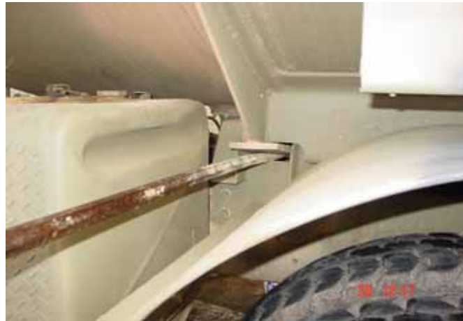
Figure 3 Crowbar Between Tank Saddle and Tank Mount – Driver Side
