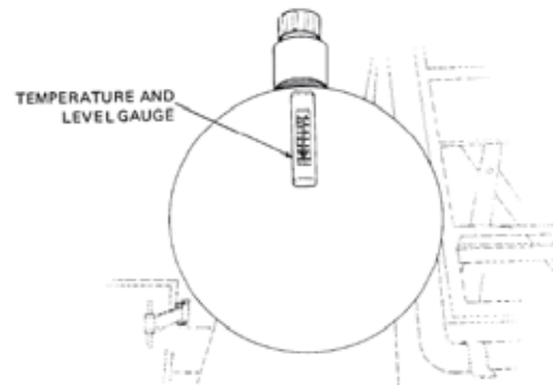
Figure 4 Oil Reservoir and Gauge
