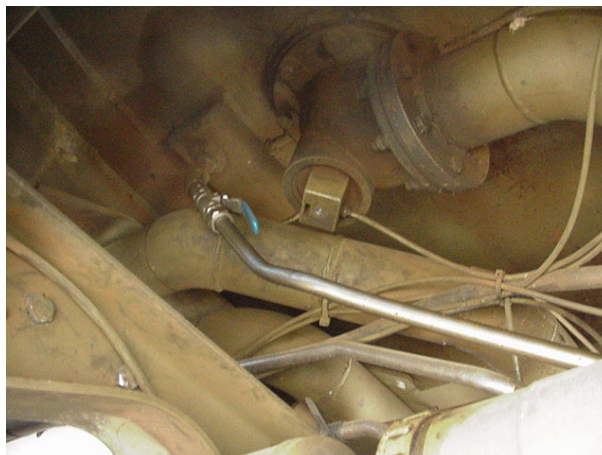
Figure 1 Forward Compartment Low-point Drain Assembly
