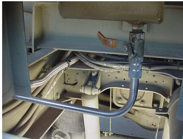
Figure 3 Rear Compartment Low-point Drain Assembly
