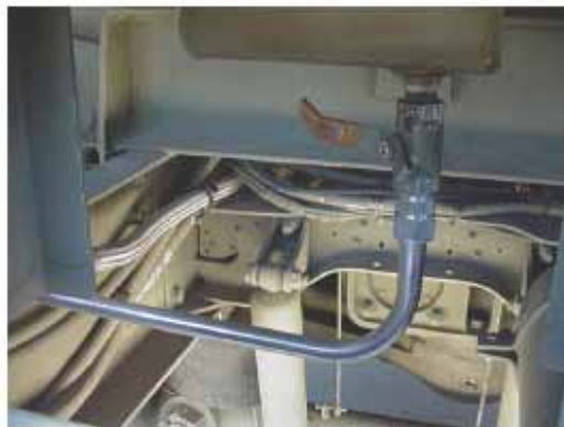
Figure 10 Rear Compartment Tank Sampling Valve Tube
