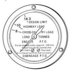
Figure 4 Load Indicator Gauge
