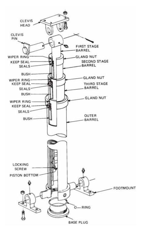
Figure 10 Hydraulic Hoist - Exploded View
