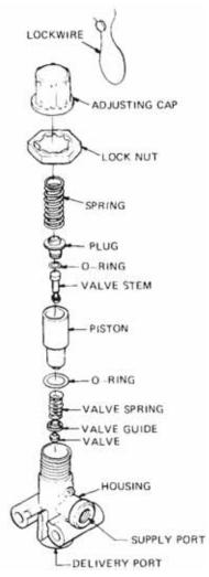
Figure 12 Pressure Protection Valve - Exploded View
