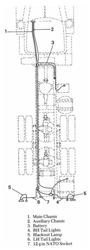
Figure 19 Rear Wiring Harness
