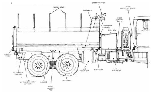
Figure 6 Dump Body and Chassis – Equipment Location
