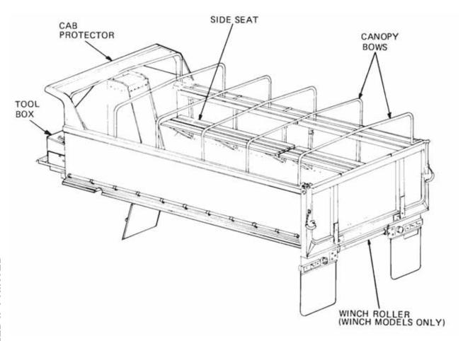
Figure 2 Dump Winch Body Assembly
