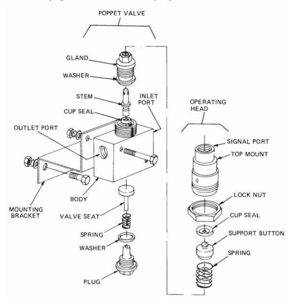
Figure 14 Poppet Valve - Exploded View
