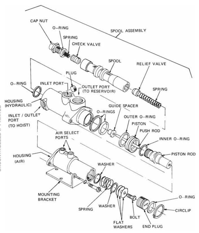
Figure 16 Hoist Control Valve - Exploded View
