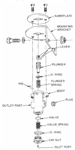
Figure 13 Tailgate Lock Valve - Exploded View
