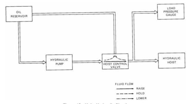
Figure 15 Hoist Hydraulic Circuit
