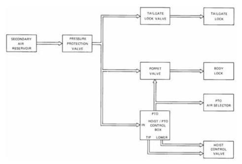
Figure 11 Air Circuit – Dump Body Lock and Hoist
