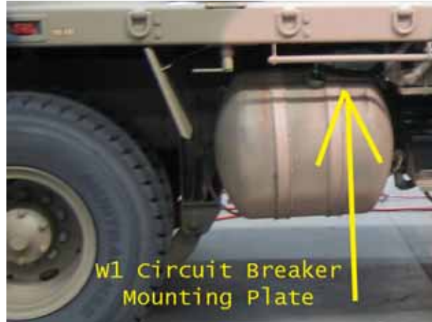
Figure 2 Location of Plate, Mounting, (W1 Circuit Breaker Box)
