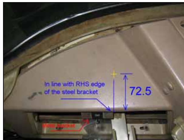
Figure 33 Centre Mark for Dashboard Cutout
