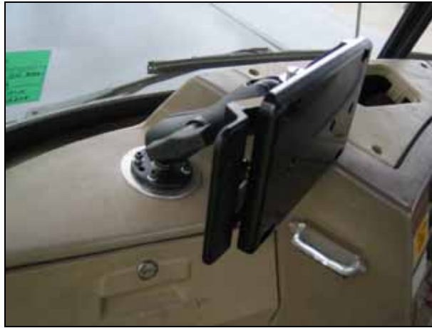
Figure 39 Chief of Section Display Mount Installed
