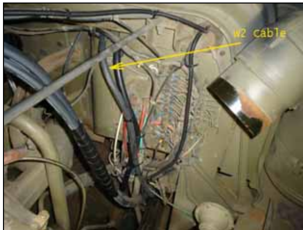
Figure 40 W2 Cable Engine Bay Installation
