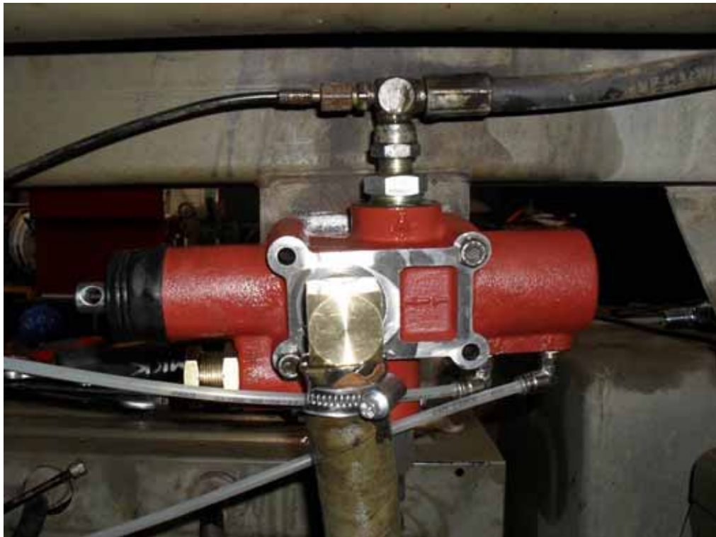
Figure 3 Position of Valve on Mounting Bracket Viewed from the Left Side of the Vehicle
