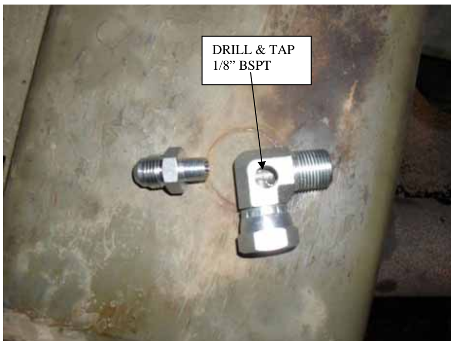
Figure 2 Modified Elbow 90 BSPT 3/8 x 3/8 Male/Female
