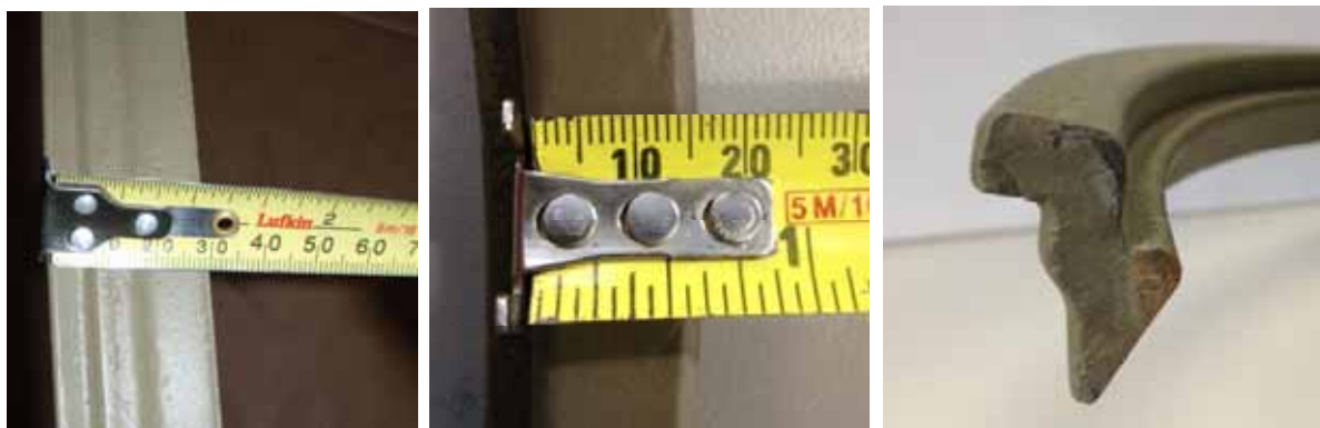
Figure 4 Mk/GKN Locking Ring – Depth (30 mm), Top (16 mm) and End Profile
