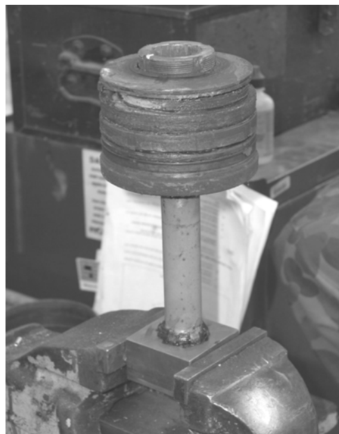
Figure 2 Torque Limiter Located In Winch Drive Shaft Securing Tool
