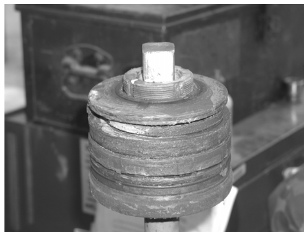
Figure 3 Winch Torque Limiter Drive Adaptor Located In Torque Limiter
