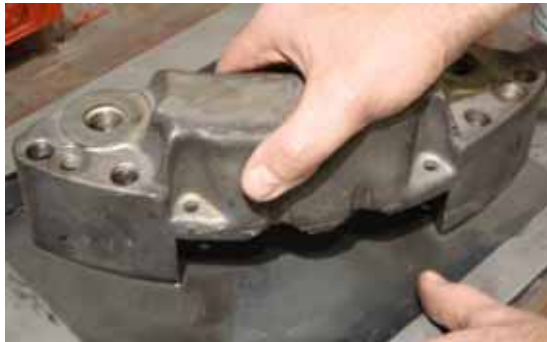
Figure 6 Surface Finishing of Machined Caliper Halves
