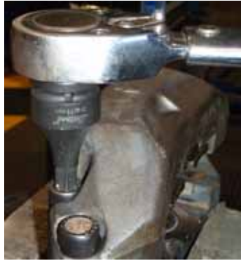
Figure 14 Applying Torque to Caliper Body Bolts
