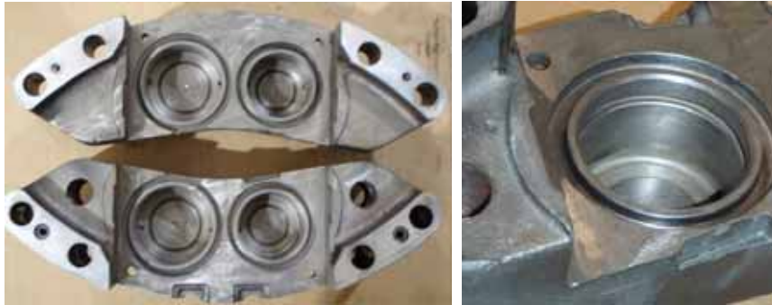
Figure 5 Piston Bores Cleaned of Residual Corrosion
