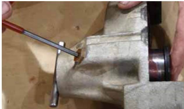
Figure 31 Winding in the Inner Piston Using Adjuster
