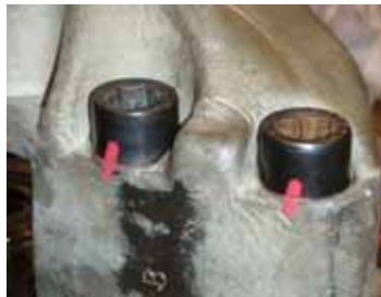
Figure 15 Witness Marking Caliper Bolts
