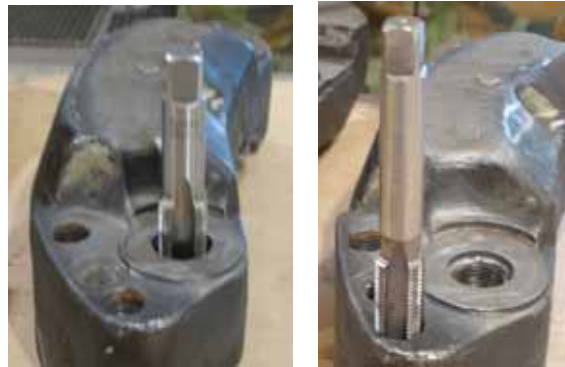
Figure 4 Confirming Threaded Holes with Suitable Taps
