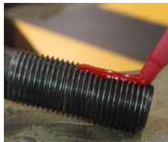
Figure 13 Applying Loctite 272 to Caliper Bolts
