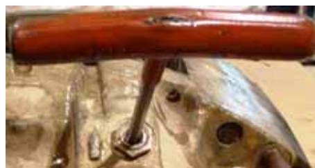
Figure 20 Cast Arrow Indicates Direction to Wind Piston out of Bore
