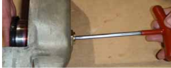
Figure 21 Winding in the Outer Piston Using Adjuster
