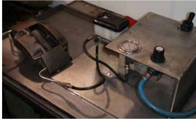
Figure 33 Pressure Testing of Brake Caliper (Front Shown)
