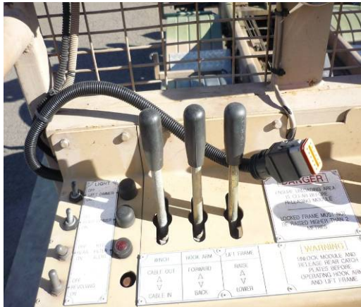
Figure 25 Harness at Control Panel
