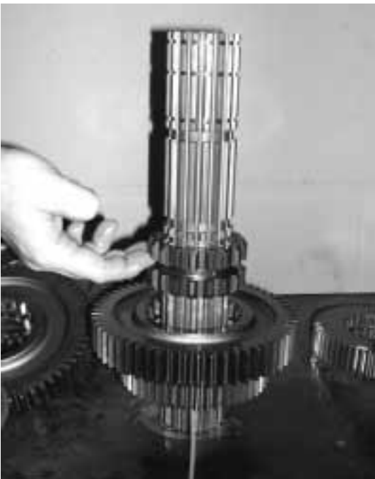
Figure 58 – Installation of 2 nd /3 rd Speed Sliding Clutch
