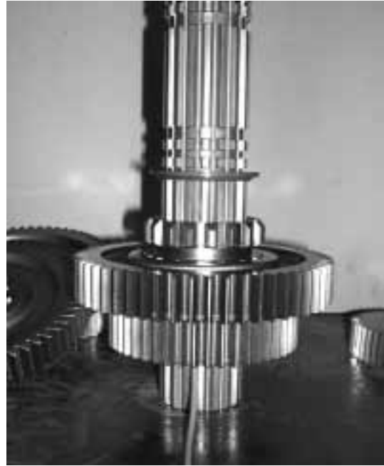
Figure 59 – Installation of 2 nd Gear Limit Washer
