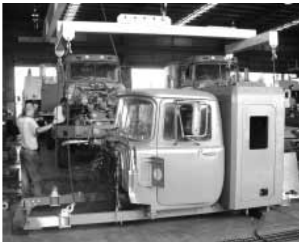
Figure 71 – Lifting Complete Cabin Assembly
