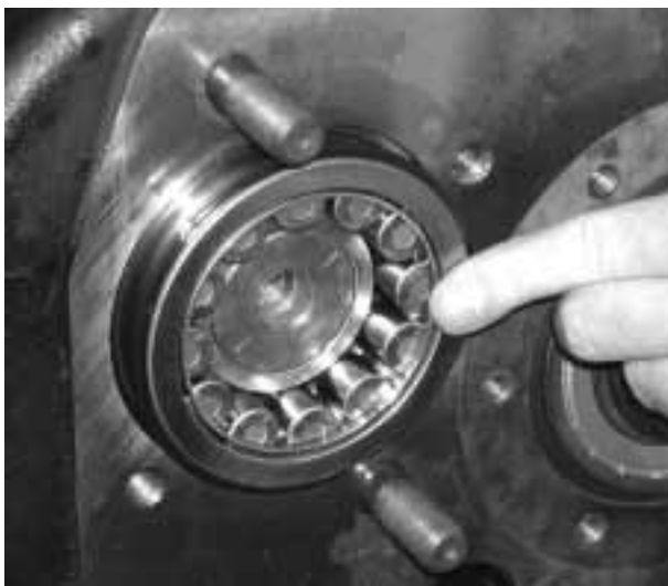
Figure 51 – Installation of Front Countershaft Bearings
