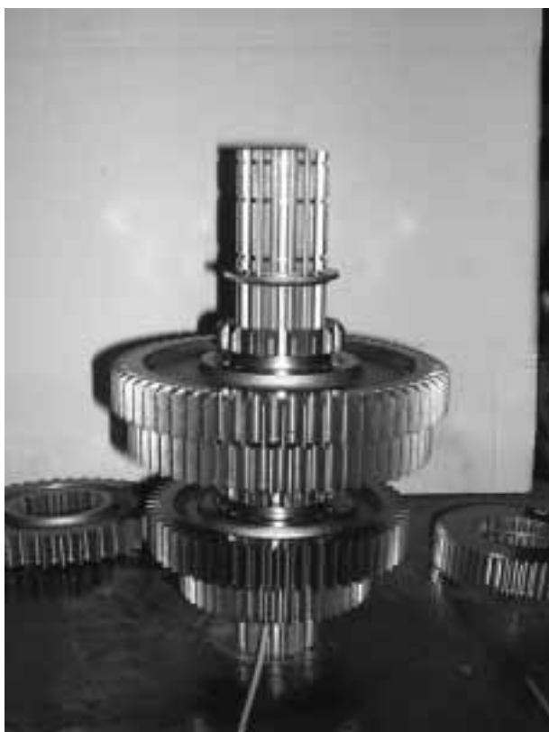
Figure 62 – Installation of Reverse Gear Limit Washer
