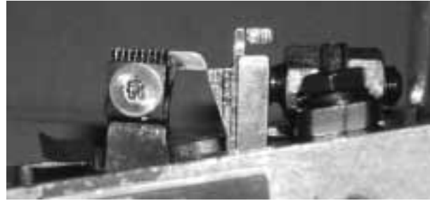
Figure 13 – Cam Nose/Stop Plate Relationship at Stop Plate Vertical Set Point
