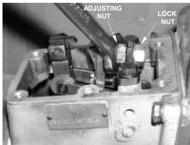
Figure 10 – Horizontal Adjustment of Stop Plate
