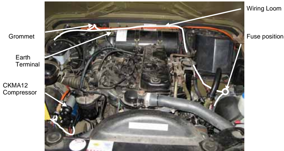
Figure 12 Engine Bay Wiring Loom
