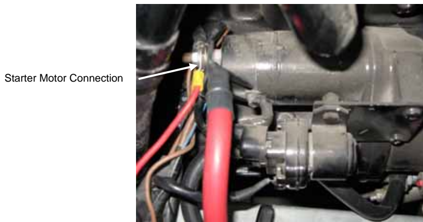
Figure 6 Starter Motor Terminal
