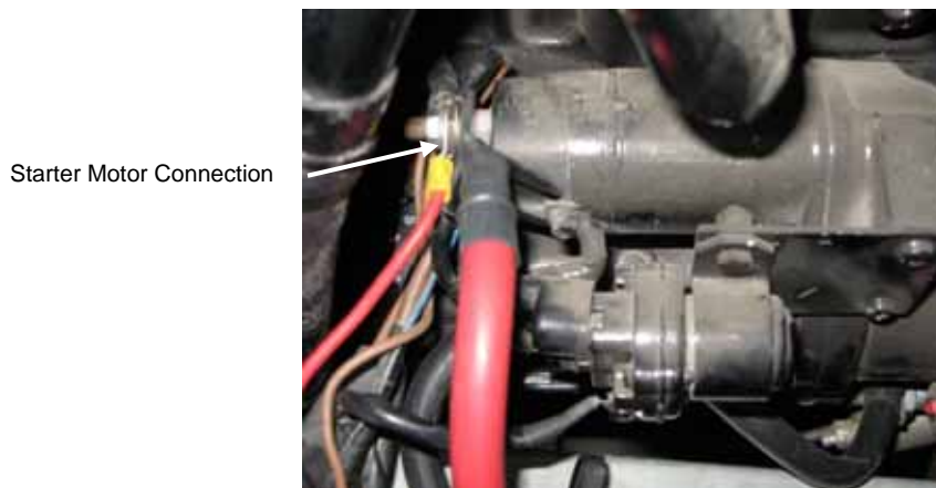
Figure 13 Starter Motor Terminal
