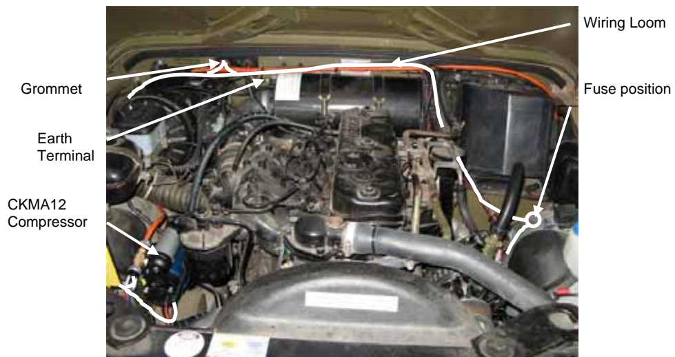
Figure 5 Engine Bay Wiring Loom
