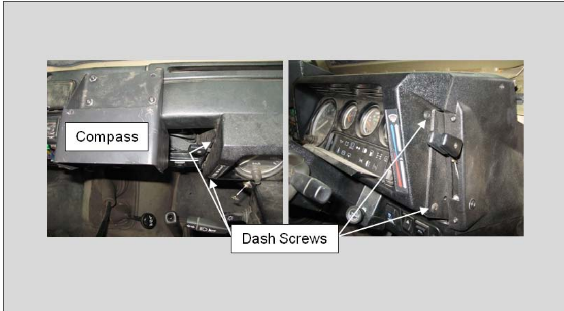
Figure 10 Partially Removed Dash
