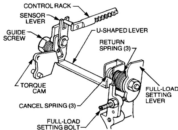
Figure 33 Full-load Setting Lever and Sensor Lever Locations
