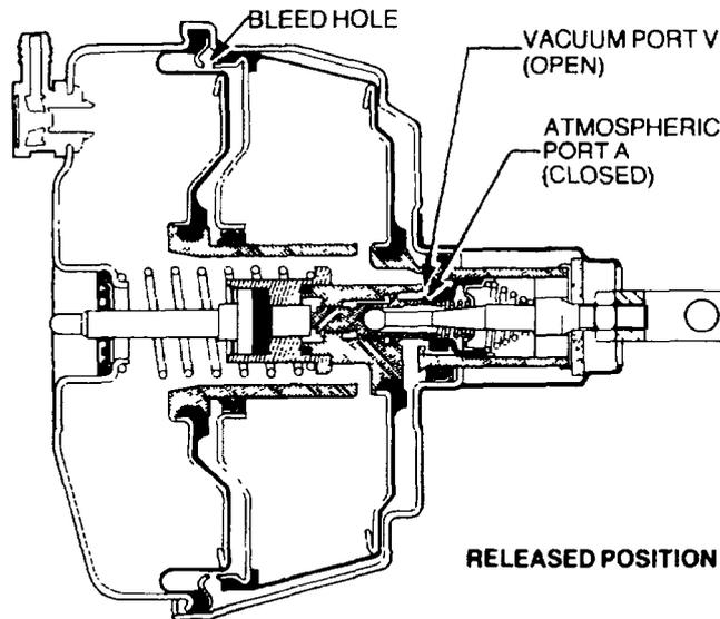
**Figure 61 Servo Diaphragms Stationary – Engine Running, Brakes Released**
