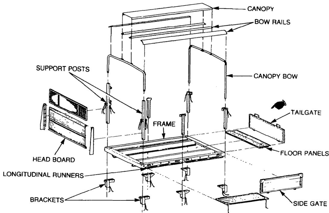
**Figure 91 Rear Body – Exploded View**
