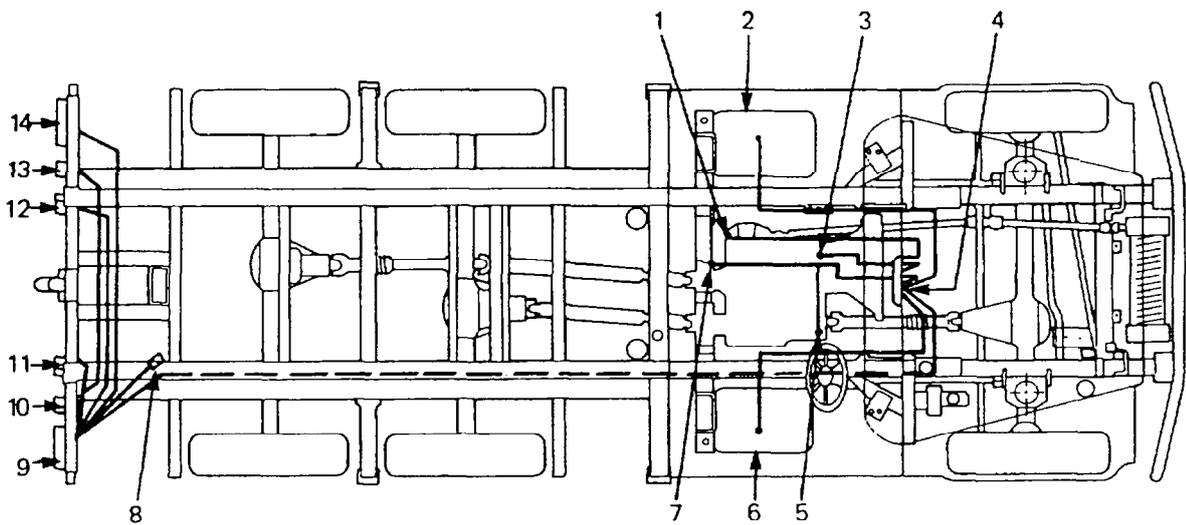
**Figure 83 Rear Wiring Harness**
