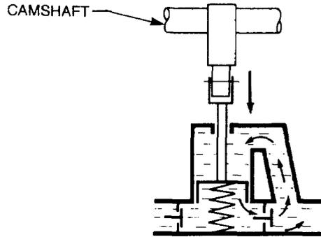
Figure 14 Discharge Stroke
