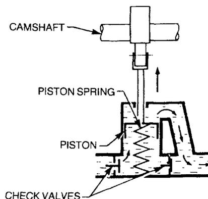
Figure 13 Intake Stroke
