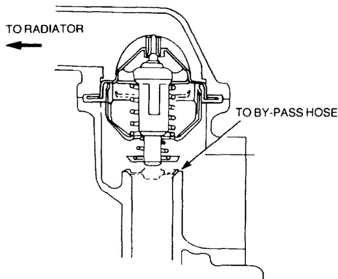
**Figure 6 Thermostat Operation**
