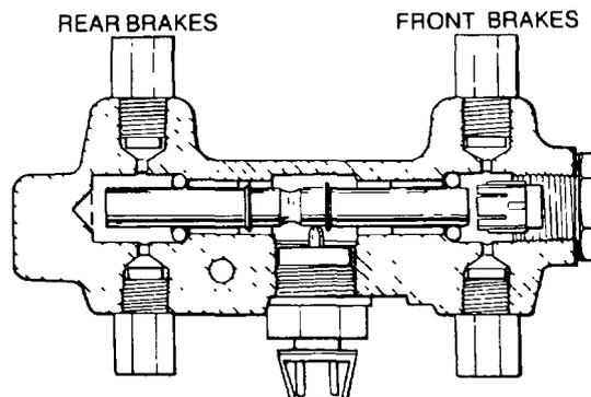
Figure 59 Hydraulic Circuit – Rear Brake Failure
