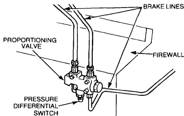
**Figure 56** Pressure Differential Switch – Location
