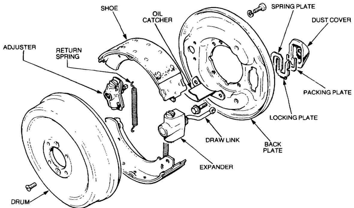
Figure 67 Parking Brake Assembly – Exploded View
