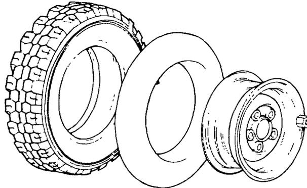
Figure 2 Tyre, Tube and Rim
