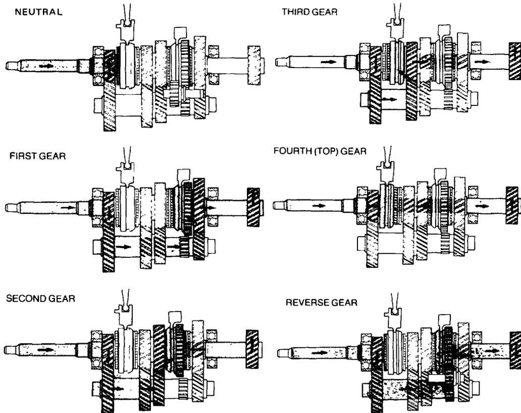
Figure 46 Drive Transmitted Through the Gears
