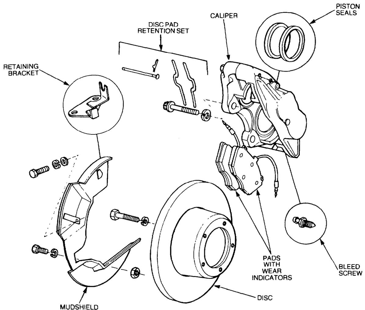
**Figure 63 Front Disc Brake Assembly – Exploded View**
