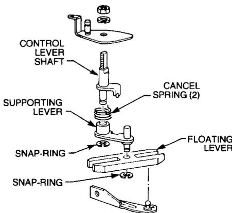
Figure 31 Control Assembly – Exploded View
