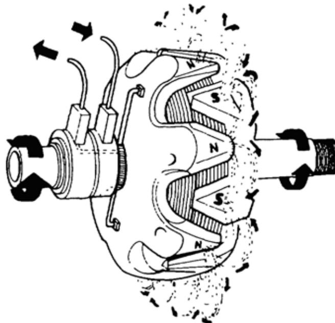
**Figure 79 Rotor and Magnetic Field**
