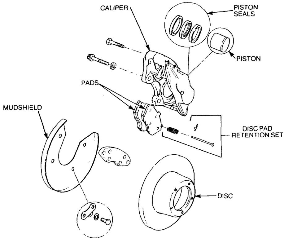
Figure 64 Rear Disc Brake Assembly – Exploded View
