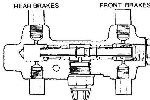
Figure 58 Hydraulic Circuit – Front Brake Failure
