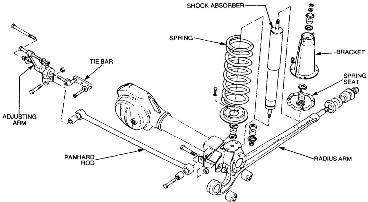
Figure 68 Front Suspension – Left-hand Side
