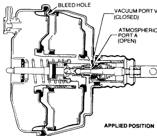
**Figure 62 Servo Chamber Operating – Brakes Applied**
