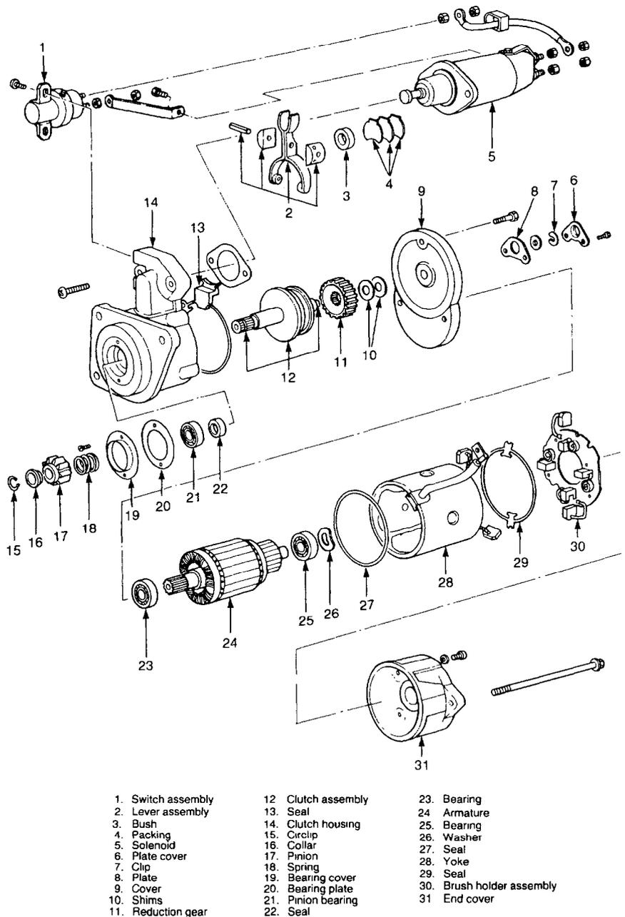
Figure 77 Starter Motor – Exploded View
