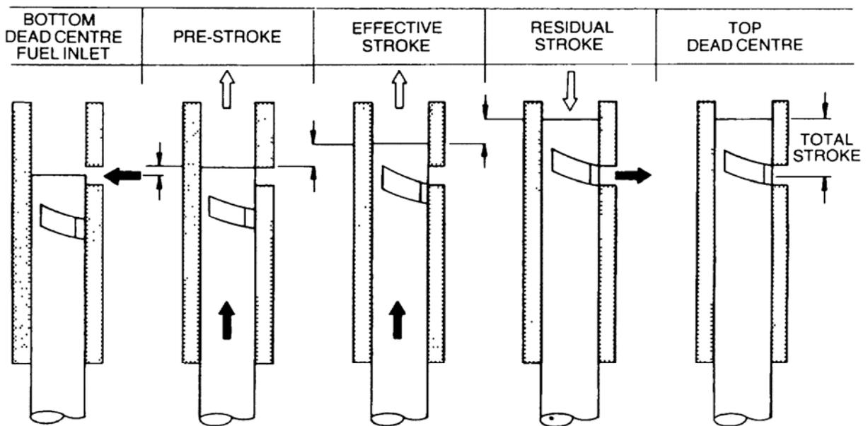
Figure 22 Phases (Strokes) of the Plunger
