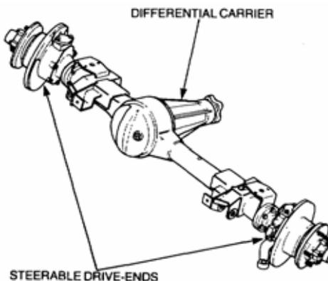
**Figure 53 Front Axle Assembly**
