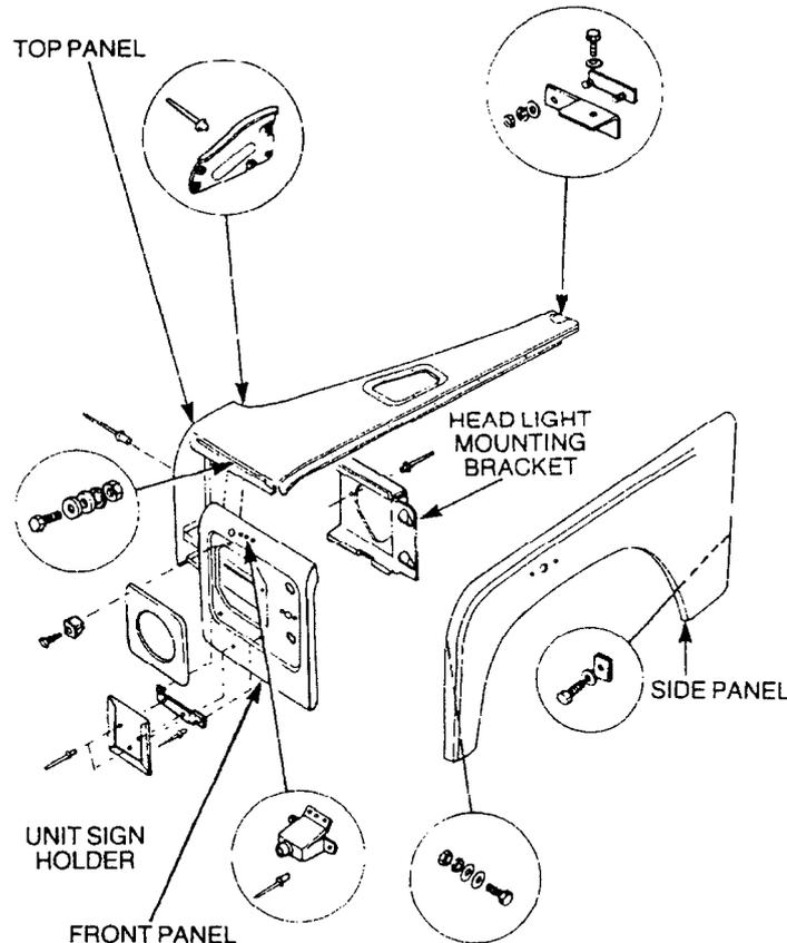
Figure 88 Left-hand Front Outer Mudguard – Exploded View
