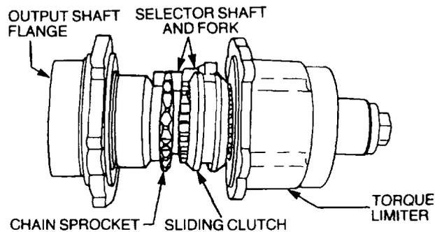
**Figure 49 PTO and Torque Limiter Assembly**
