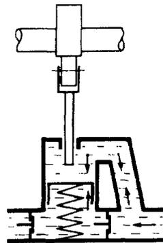
Figure 15 Pump Pressure Regulating
