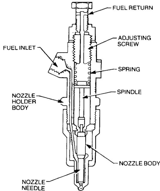
Figure 23 Fuel Injector Assembly
