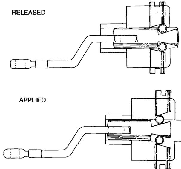
Figure 66 Parking Brake Expander Operation
