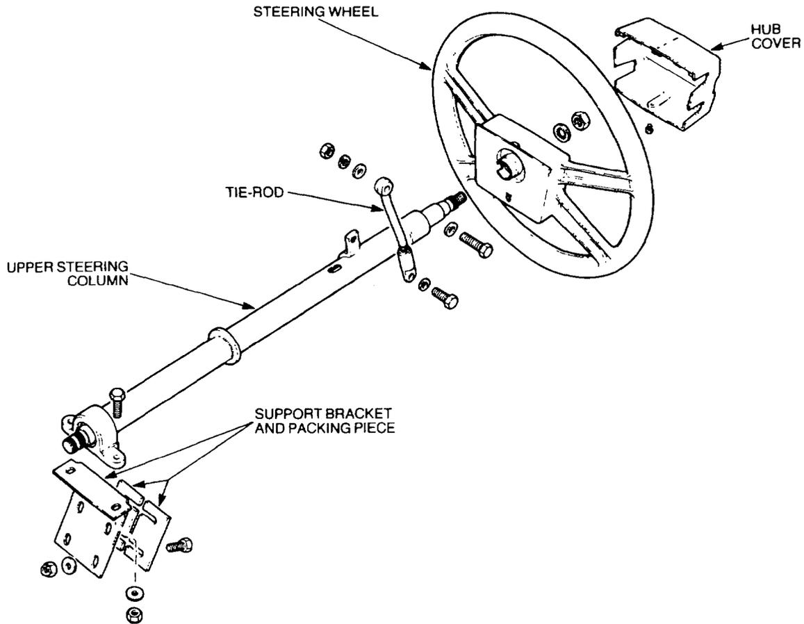
**Figure 70 Steering Wheel, Column and Upper Shaft Assembly**
