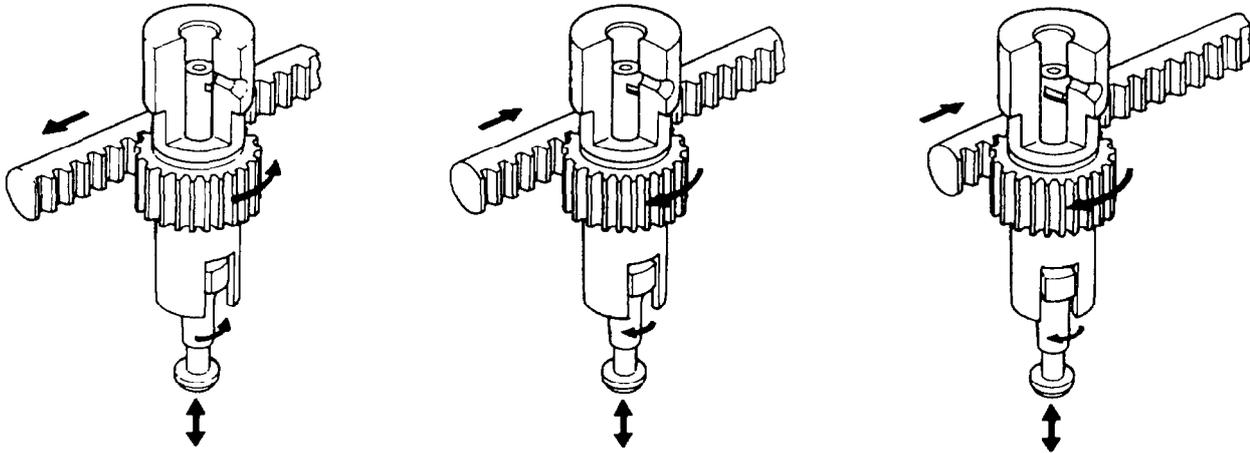
Figure 19 Plunger Rotating Mechanism
