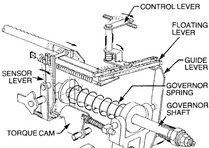
Figure 36 Returning to the Idle Position
