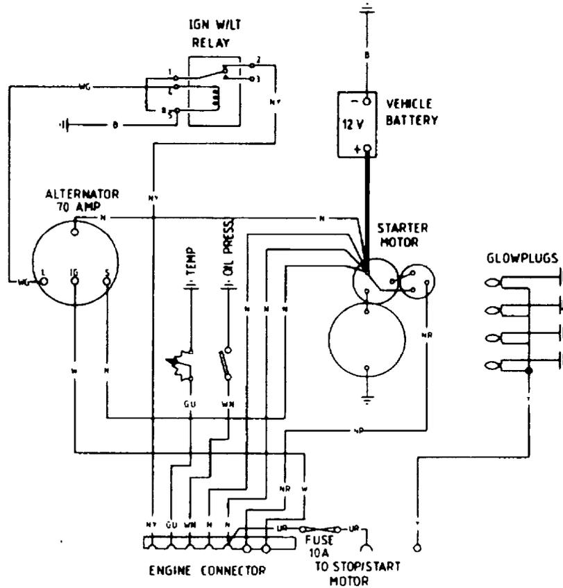
Figure 74 Engine Electrical Circuit
