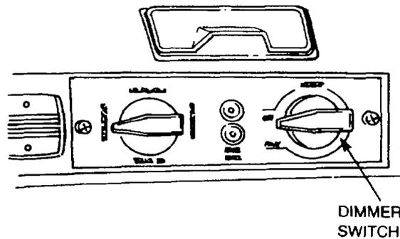
Figure 81 Lighting Control Switch Location
