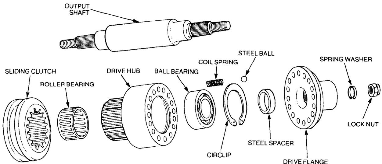
**Figure 50 Torque Limiter and Output Shaft – Exploded View**
