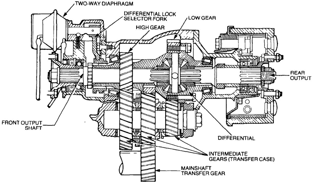
Figure 47 Transfer Case and Differential – Sectional View
