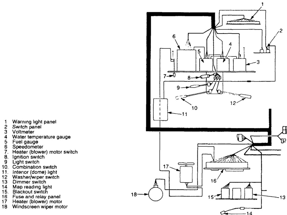
Figure 84 Cabin Wiring
