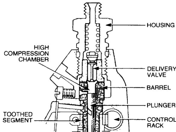
Figure 21 Housing and Delivery Valve Location
