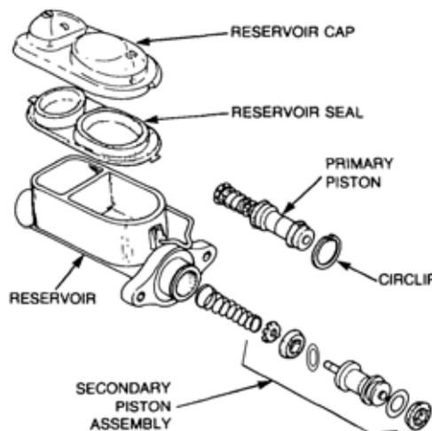
Figure 55 Dual Master Cylinder – Exploded View
