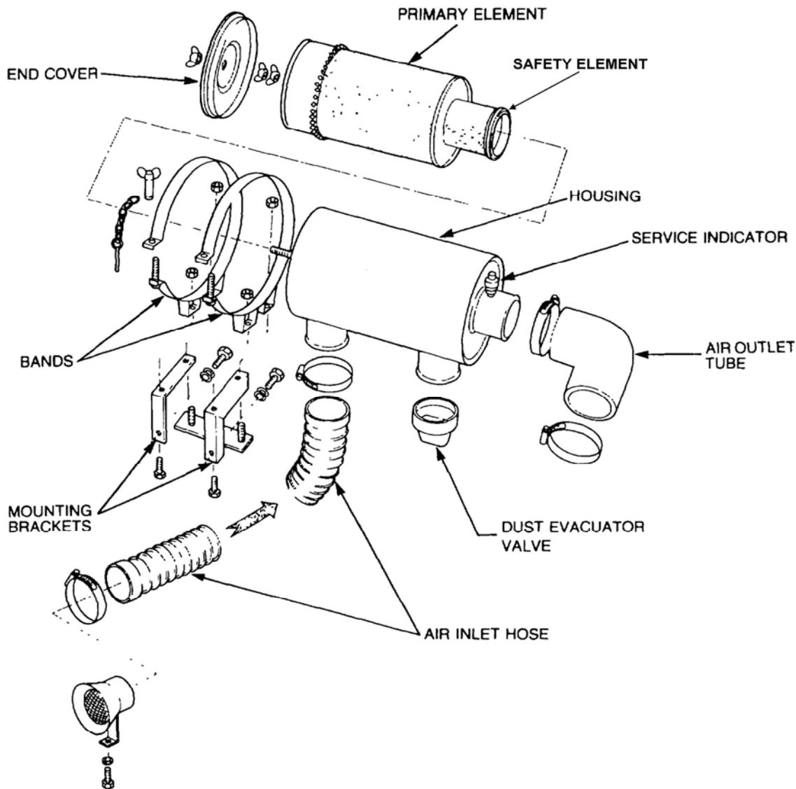
Figure 9 Air Cleaner Assembly – Exploded View
