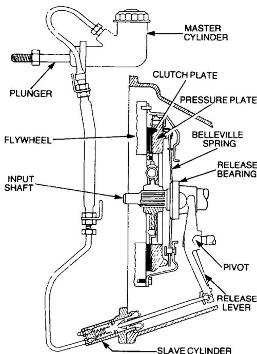
**Figure 44 Clutch Assembly – Sectional View**
