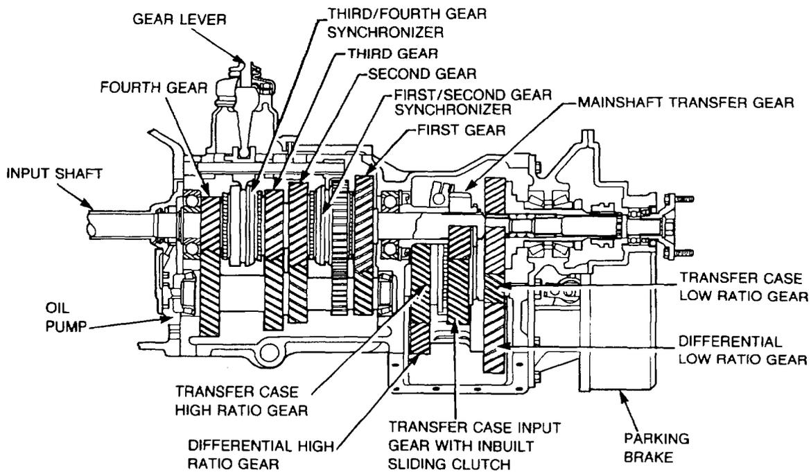
Figure 45 Transmission Assembly – Sectional View
