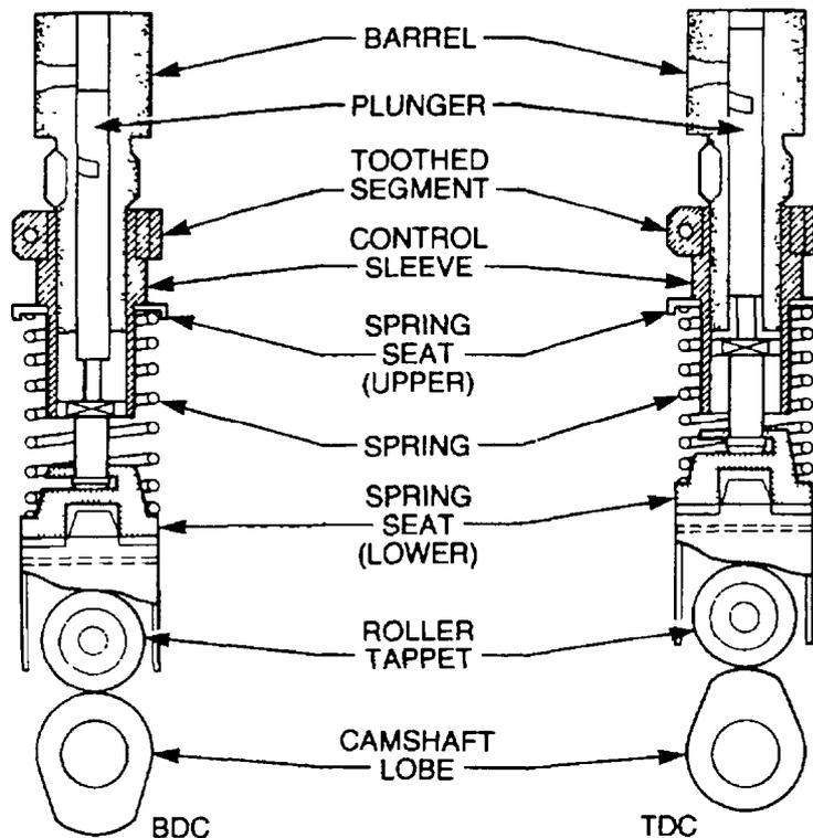
Figure 20 Plunger Drive Assembly
