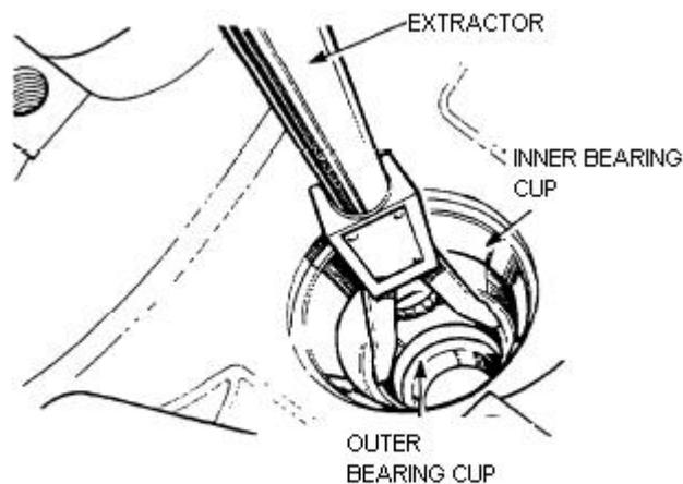
**Figure 209 Removing the Pinion Bearing Cup**
