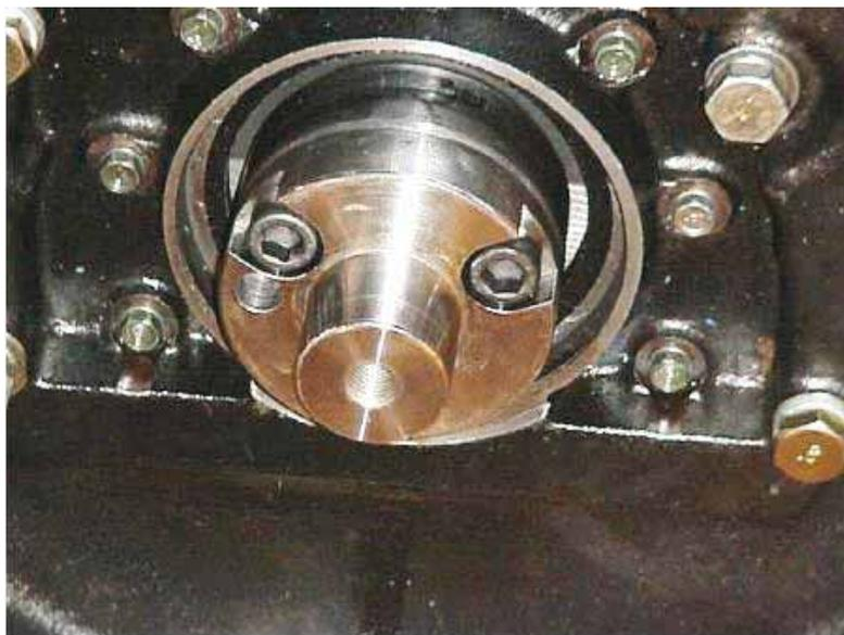
**Figure 47 Crank Plate Secured to Crankshaft**
