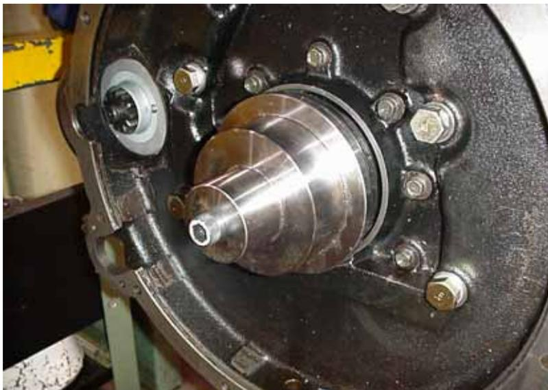
**Figure 49 Push Cone Located on Crank Plate and Against Seal**
