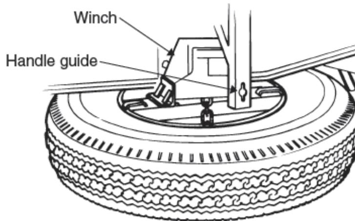
Figure 22 Spare Wheel Winch Mounting
