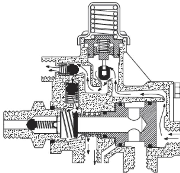
Figure 9 SR3 Spring Brake Control Valve – Charging
