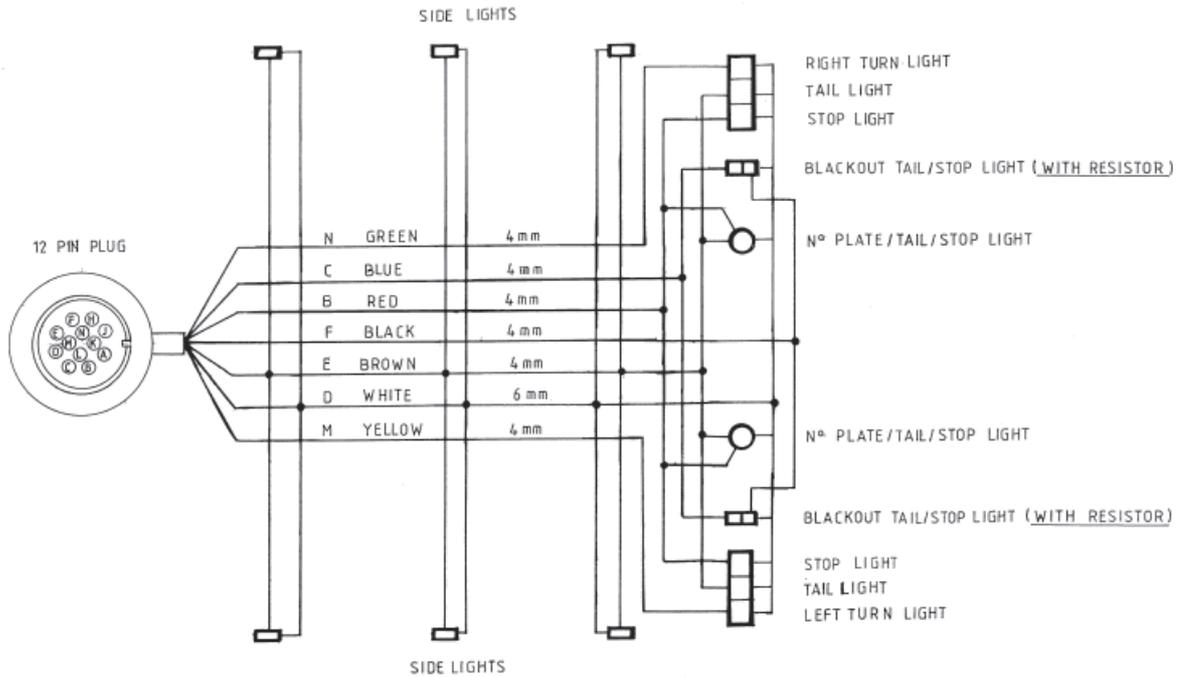
**Figure 19 Electrical Circuit Diagram – Version 1**
