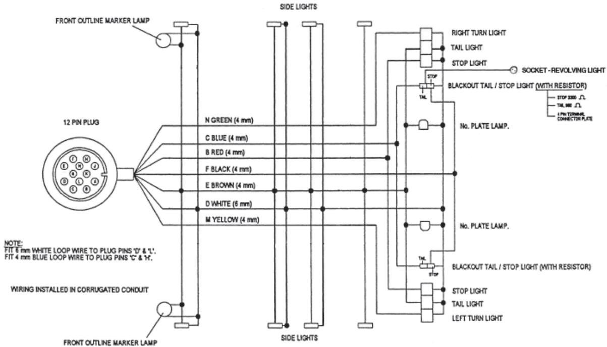
Figure 21 Electrical Circuit Diagram – Version 4
