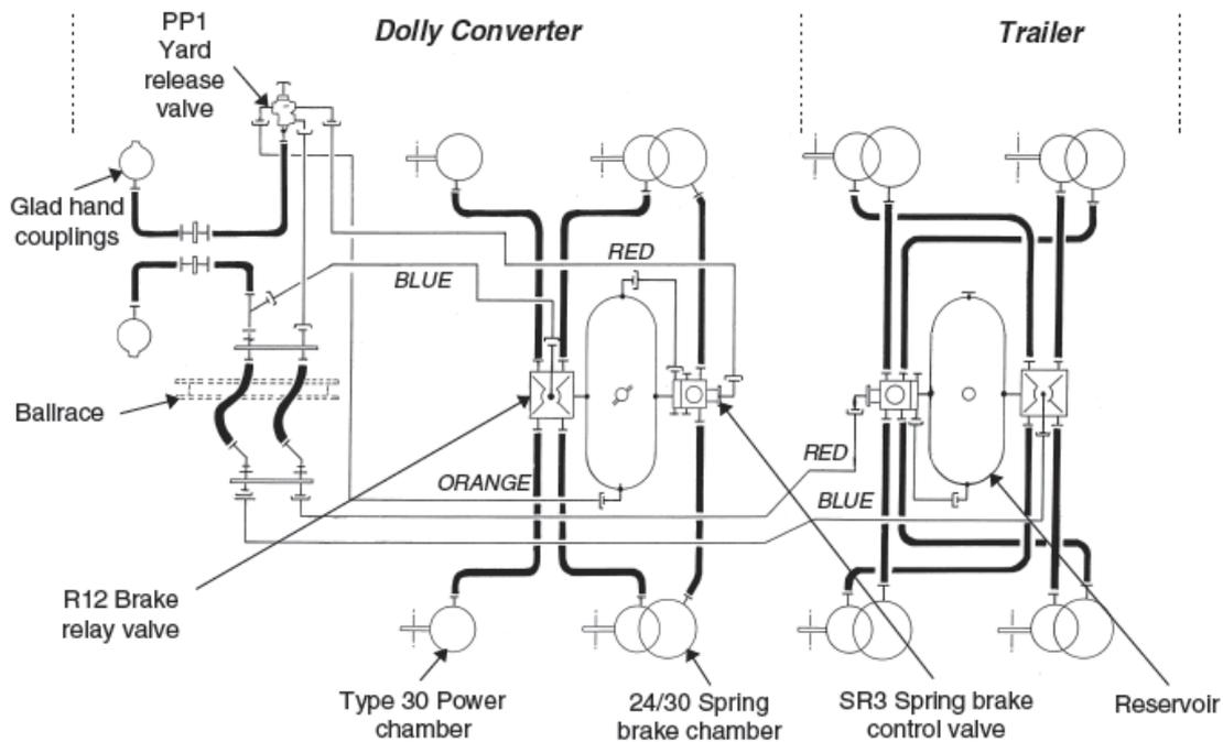
**Figure 1 Trailer Versions 1, 2 & 3 Brake System – Westinghouse**
