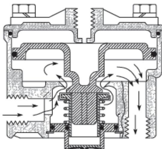
**Figure 6 Brake Relay Valve – Applying**
