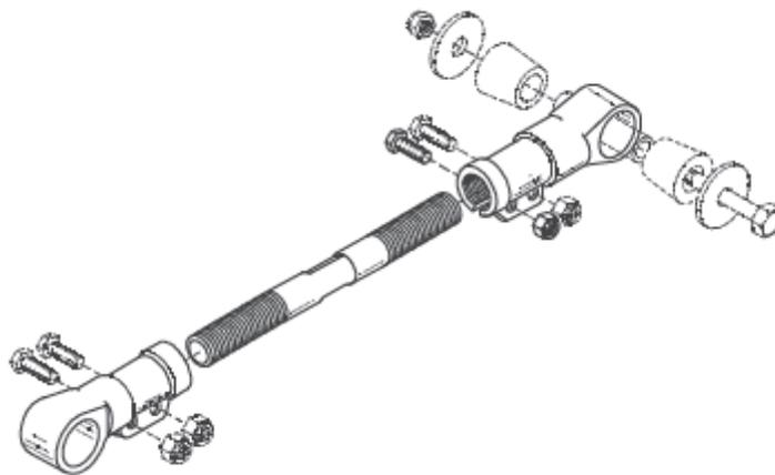
Figure 18 Adjustable Length Radius Rod
