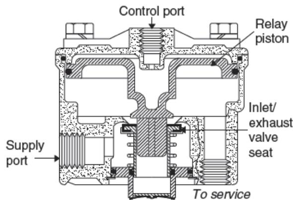
Figure 3 Brake Relay Valve – Cross Sectional View
