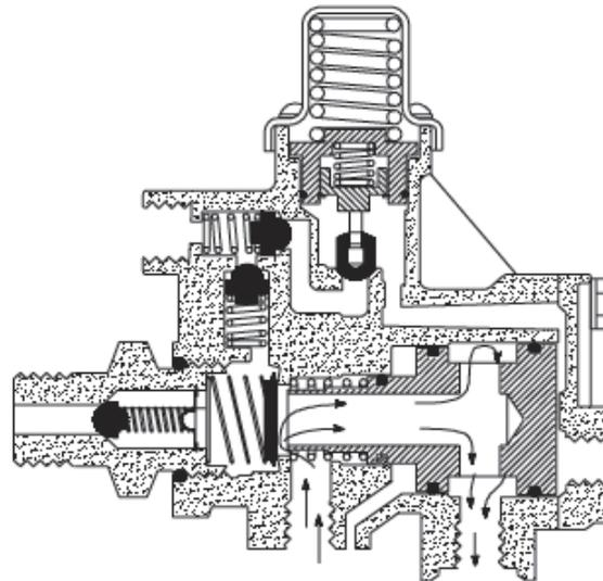
Figure 10 SR3 Spring Brake Control Valve – Park Application
