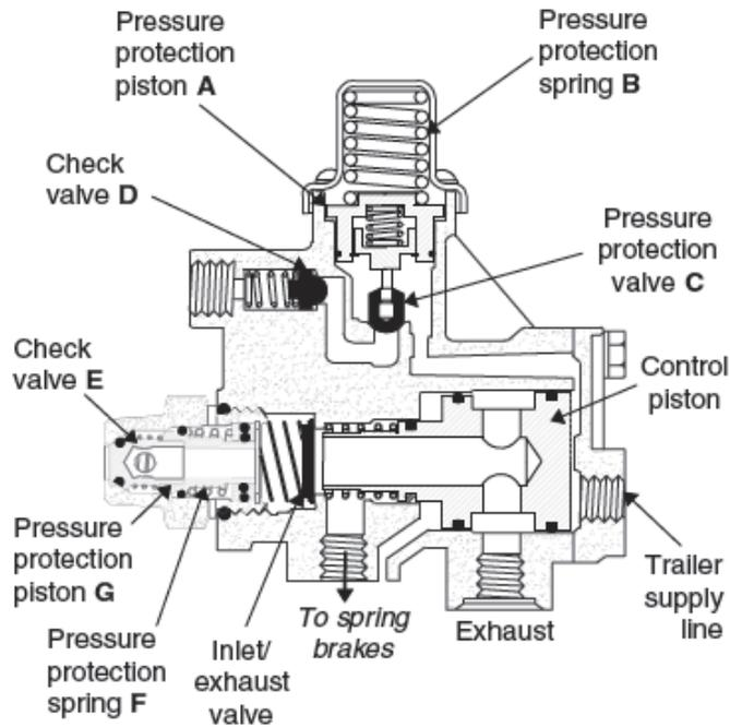
**Figure 5 ABV3802 Spring Brake Control Valve – Cross Sectional View**
