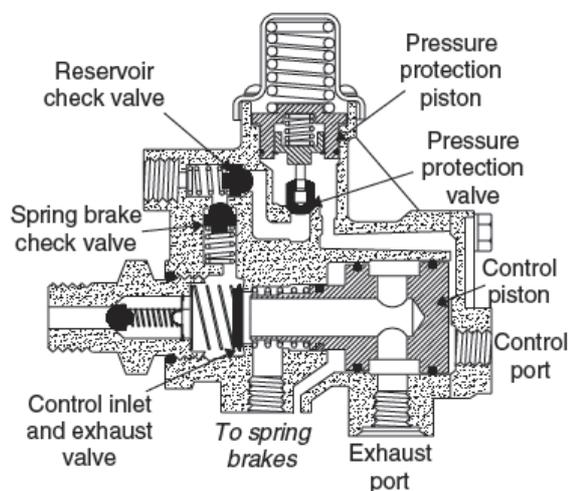
Figure 4 SR3 Spring Brake Control Valve – Cross Sectional View
