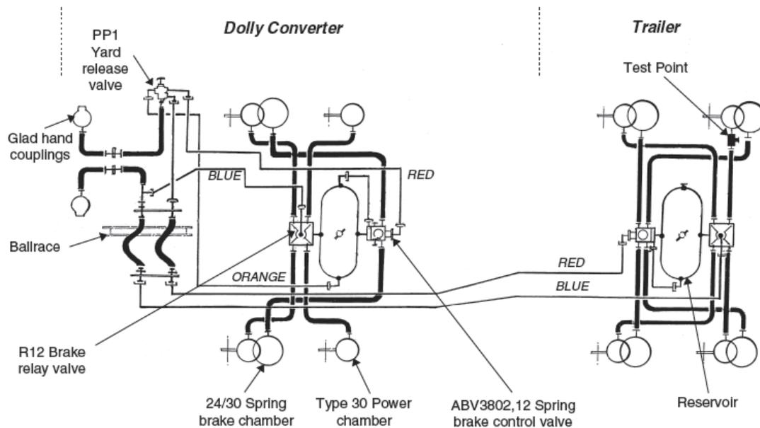
**Figure 2 Trailer Version 4 Brake System – Air Brake Corporation**
