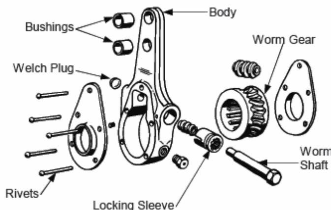
Figure 15 Slack Adjuster Assembly – Exploded View
