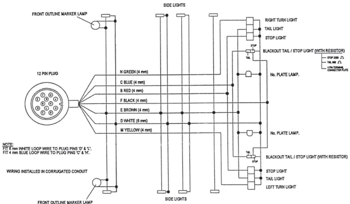
**Figure 20 Electrical Circuit Diagram – Versions 2 & 3**
