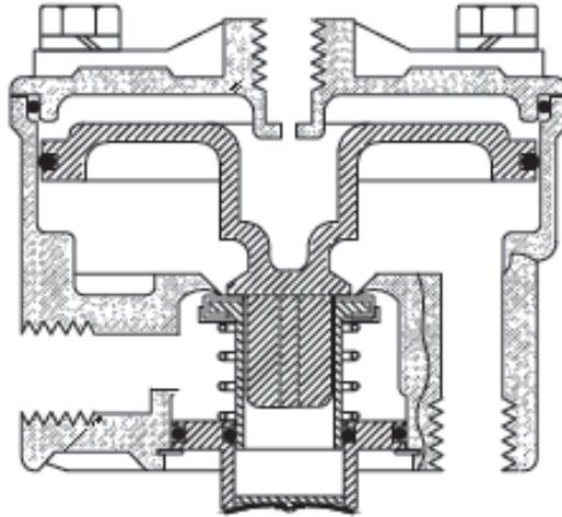
Figure 7 Brake Relay Valve – Balanced Position
