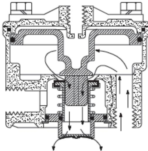
Figure 8 Brake Relay Valve – Releasing
