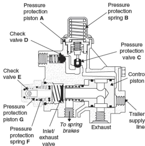
Figure 12 AB3802 Spring Brake Control Valve – Cross Sectional View
