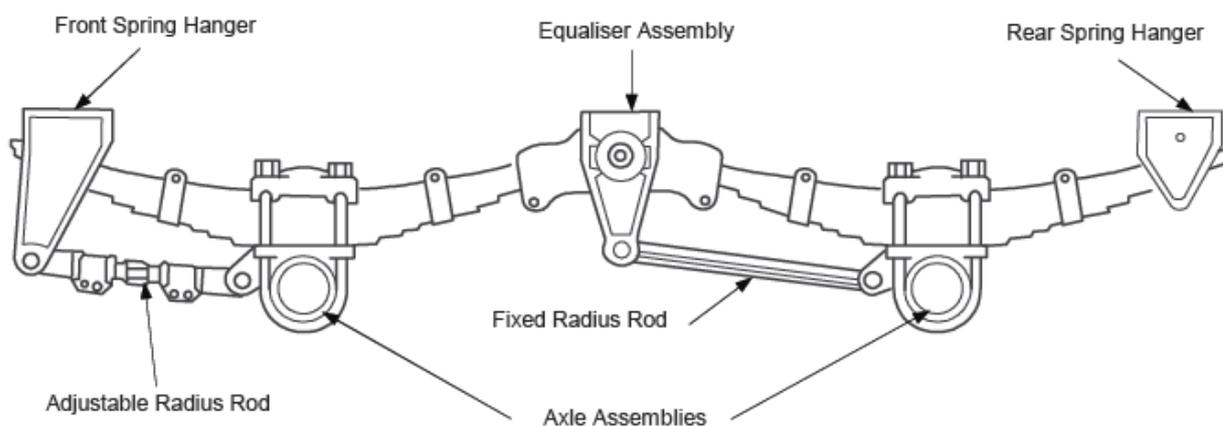
Figure 16 Trailer Suspension Layout
