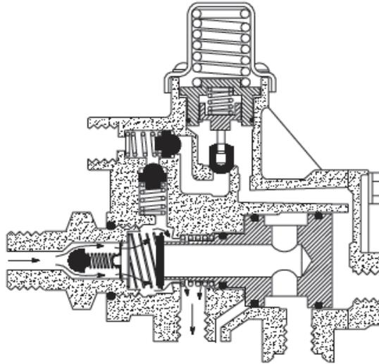
Figure 11 SR3 Spring Brake Control Valve – Brake System Failure
