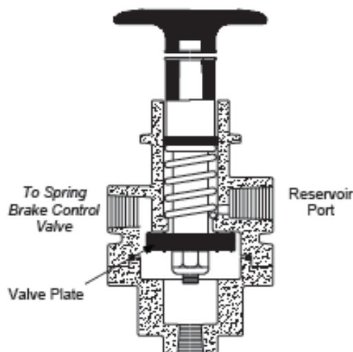
Figure 13 Yard Release Valve – Cross Sectional View
