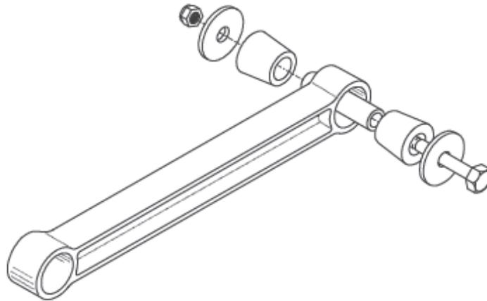
Figure 17 Fixed Length Radius Rod
