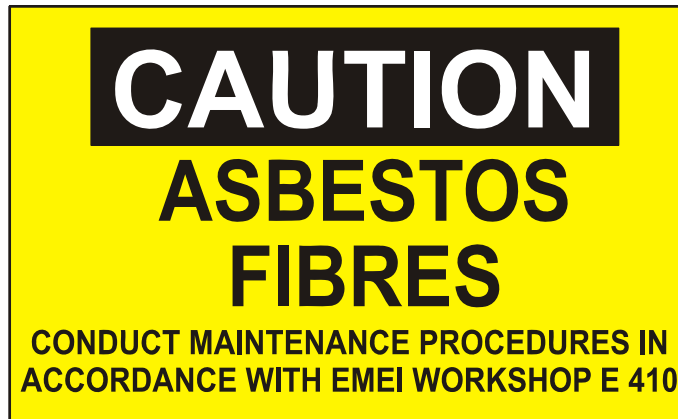
Figure 2 Adhesive Label Equipment – Asbestos Caution – 90 mm by 55 mm (Shown Actual Size)
