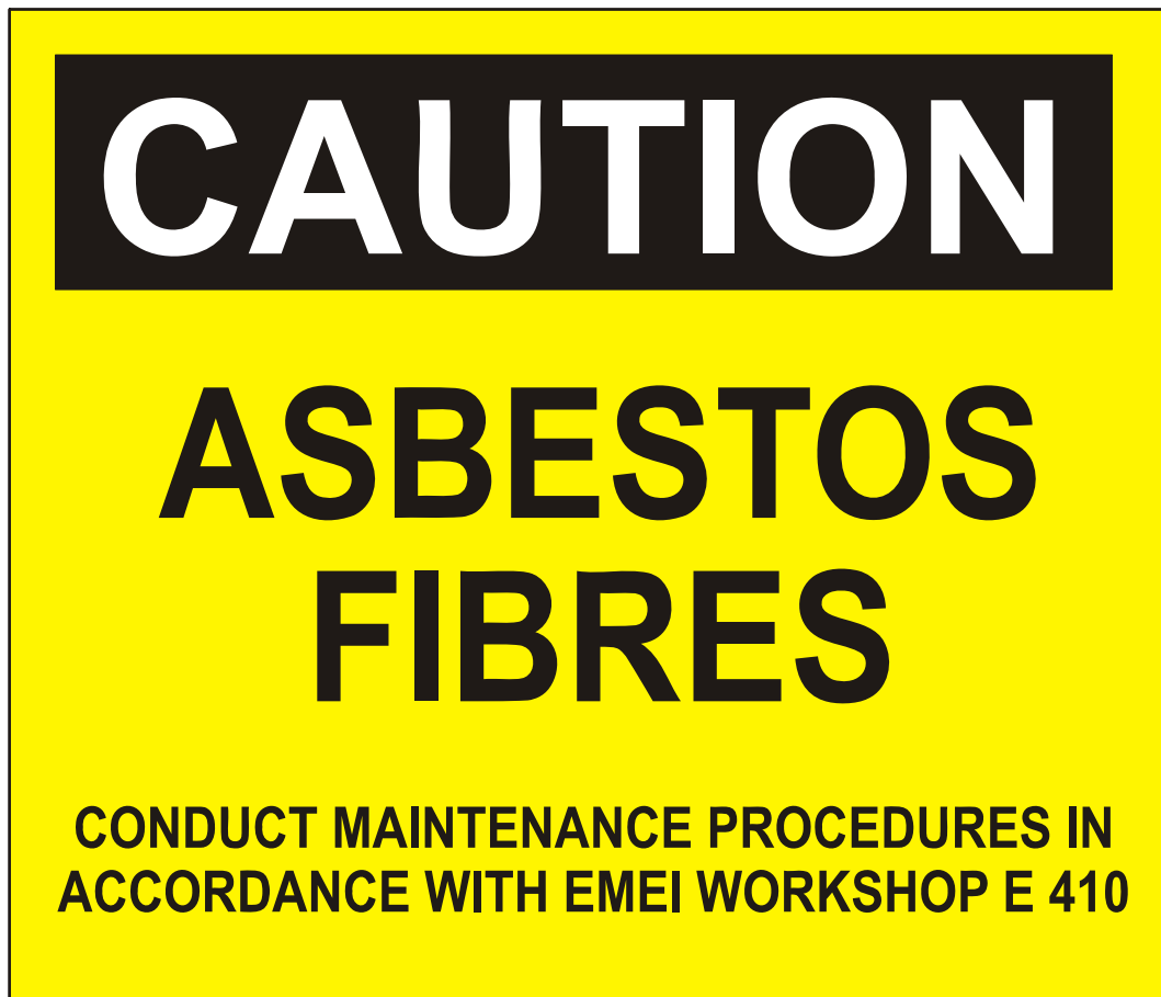
Figure 3 Adhesive Label Equipment – Asbestos Caution – 140 mm by 120 mm (Shown Actual Size)
