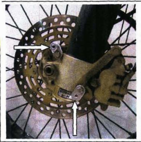
Figure 1. Mounting brackets in position. Bracket with long boss goes to top, boss facing outwards. Bracket with short boss goes to bottom, boss facing inwards
