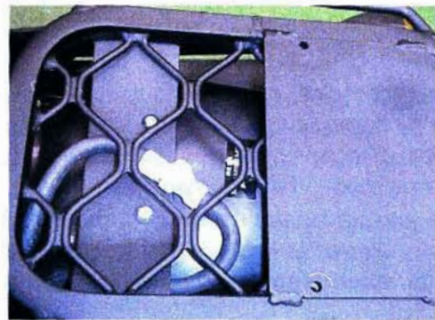
Hoses Interconnected after Tank Removal
