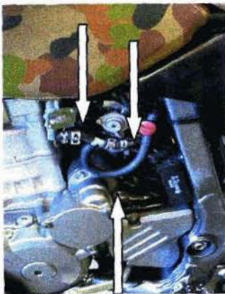
Disconnect Fuel Hoses
