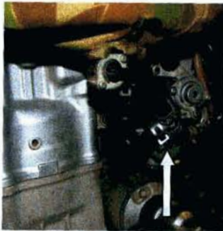
Fuel lines connected to tee
