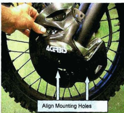
Fig 3. Offering Disc Protector to Mounting Brackets
