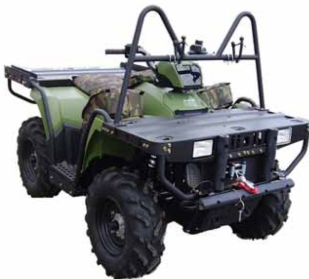
Figure 1 All Terrain Vehicle, Polar is 4x4 Sportsman 700 Military Variant (MV 7 ), With Winch.
