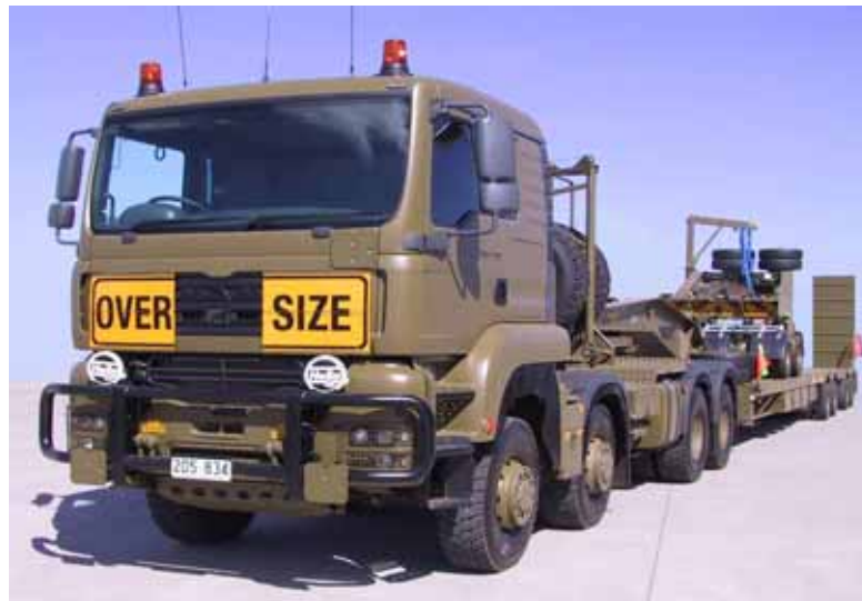
Figure 1 Truck Tractor, Heavy Tank Transporter, MC3, MAN 8X8 Prime Mover, 6 Cylinder Diesel Engine, 12 Speed TC-Tronic
