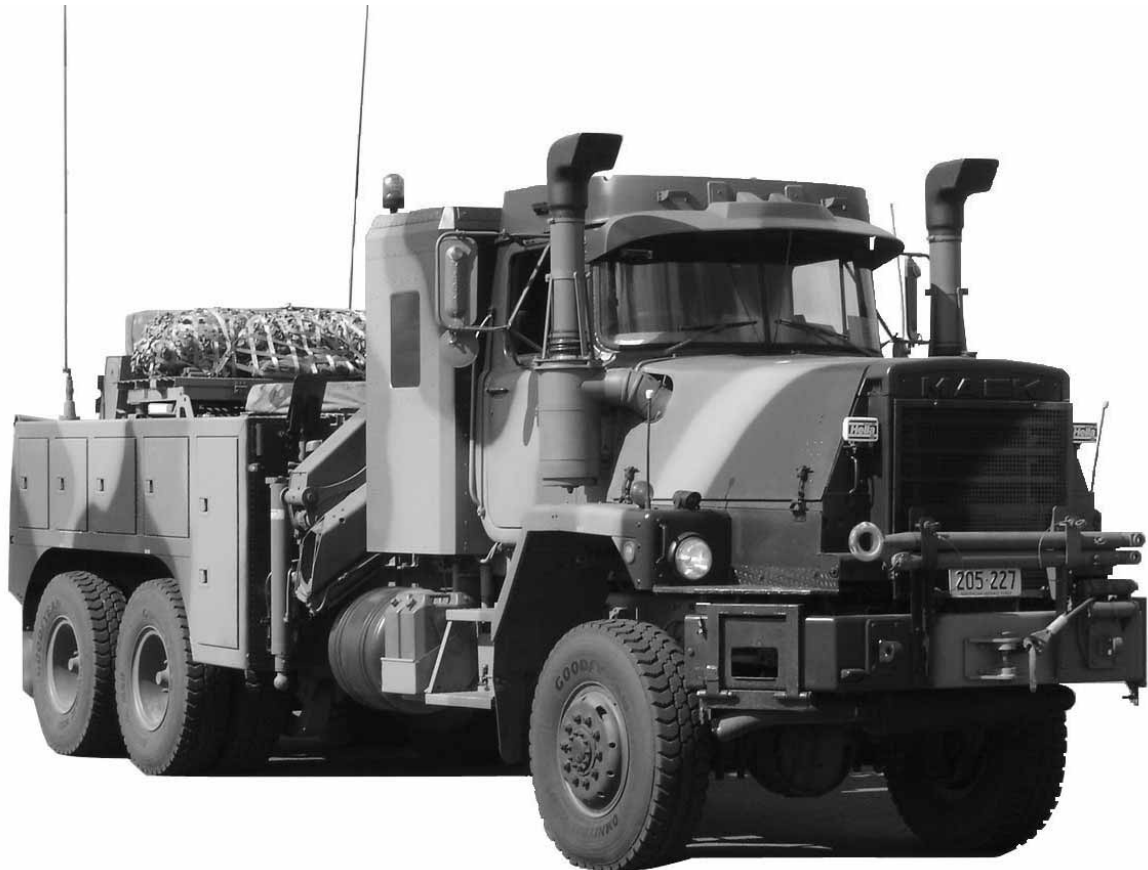
Figure 1 Truck, Wrecker, Heavy Recovery Vehicle (HRV), MC3, 123T GCM, 6X6, HYDRAULIC Lift/Tow, W/Twin Winch, Palfinger Crane, Mack 'R' Series
