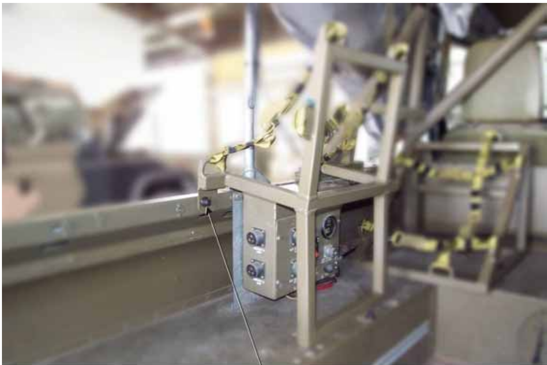
Figure 15 Combat Pack Frame Mounting Points
