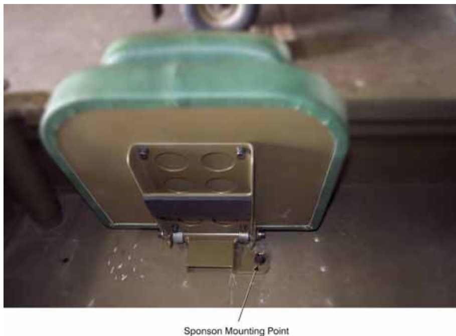
Figure 19 Operator Seat Sponson Mounting Point
