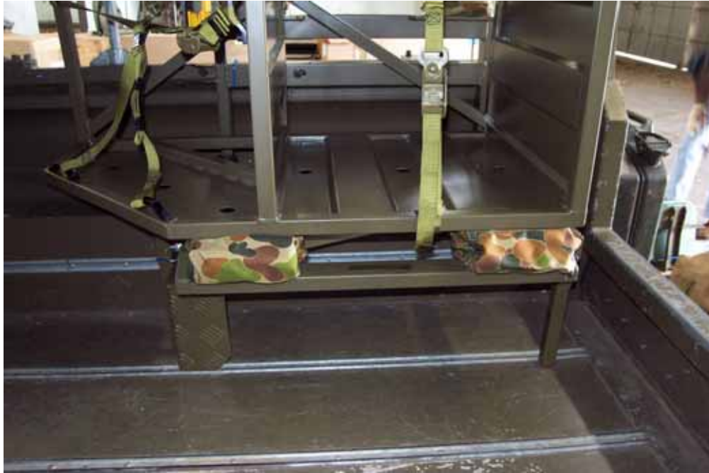
Figure 6 Vibration Isolator Covers Fitted (Front)
