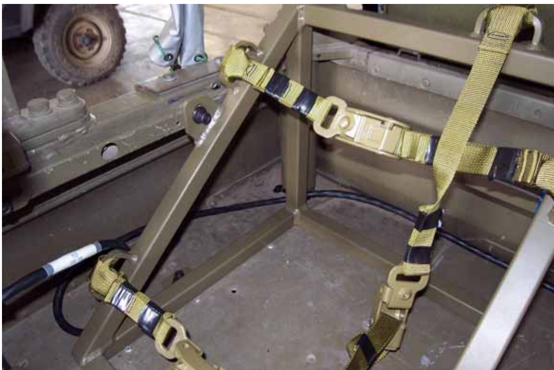
Figure 9 Vehicle Power Cable Routing
