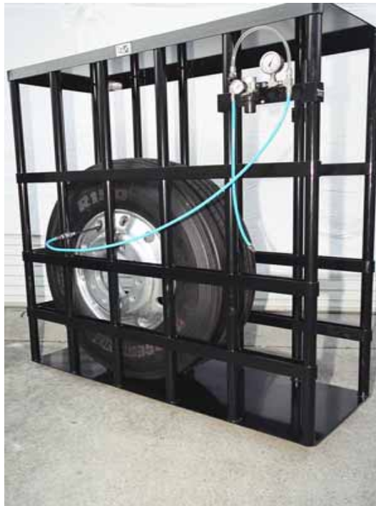
Figure 23 Tyre Inflation – Safety Cage
