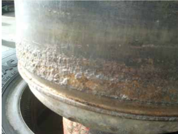
Figure 13 Severely Corroded Wheel Rim
