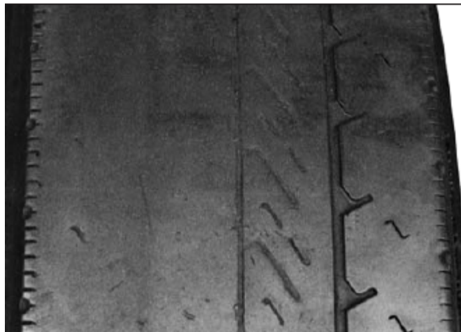
Figure 9 Wear Pattern – Excessive Camber
