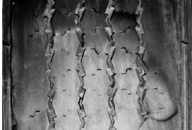
Figure 8 Spot or Cupping Wear
