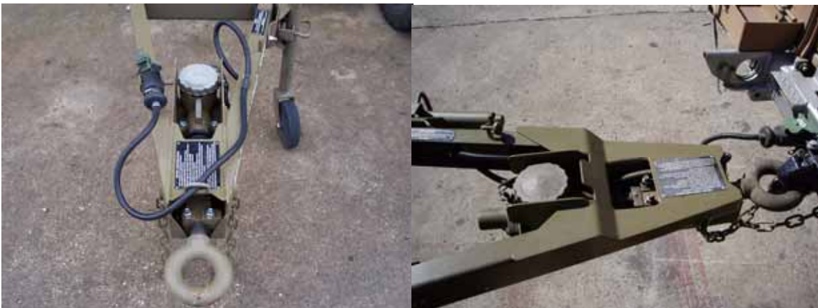
Figure 1 Original and Modified Tow Coupling Assembly and 'A' Frame Configuration
